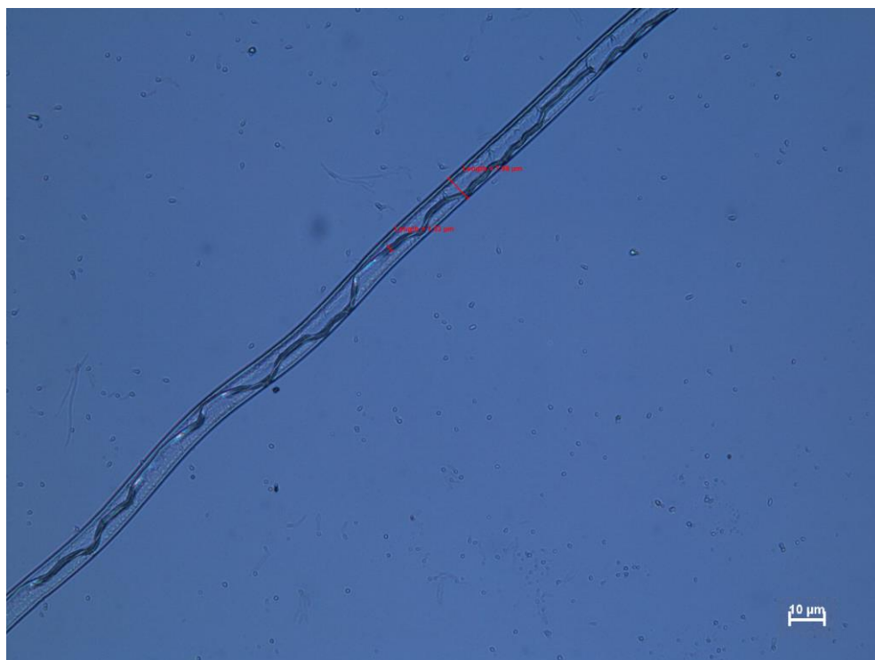
Figure 4.13. Core-shell structure of CS1 membrane
