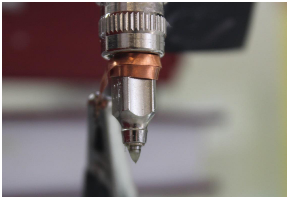
Figure 4.1. Photograph of a stable Taylor cone
