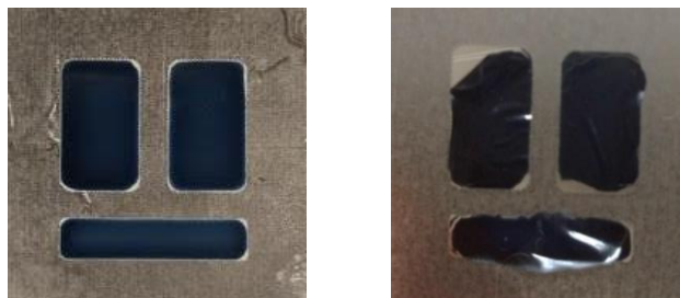
Figure 3.1 Difference between corona treated vs. non-treated PET substrates
