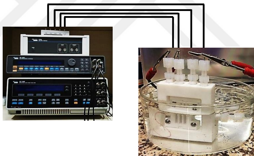
Figure 2.5 Conductivity cell set-up system connected to Solartron 1260&1278A. OEIP system inserted into conductivity cell is plunged into deionized water bath for measurement
