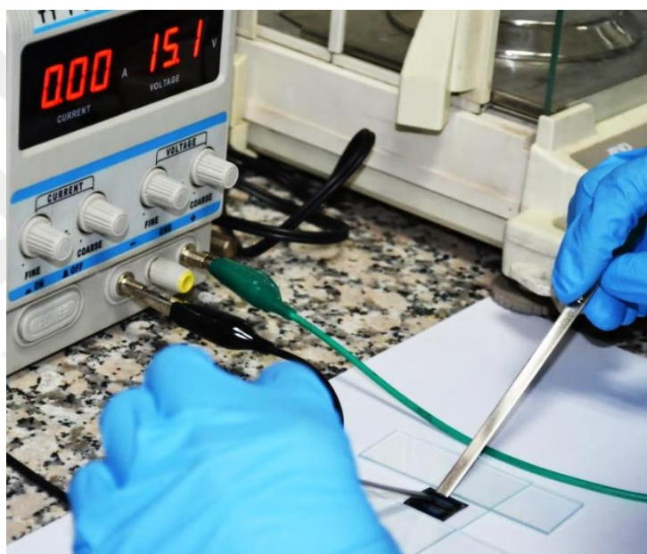
Figure 2.2 Overoxidation step of PEDOT:PSS electrodes. A pre-determined 2 mm region is electrochemically overoxidized with 20% KCl solution via applied voltage
