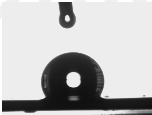
Figure 3.2 : Photograph from contact angle measurement of AAM after ODTS coating.
