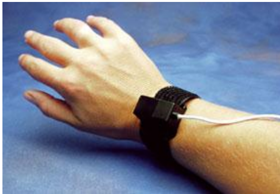
Figure 10.a) A tri-axial accelerometer mounted on wrist and
