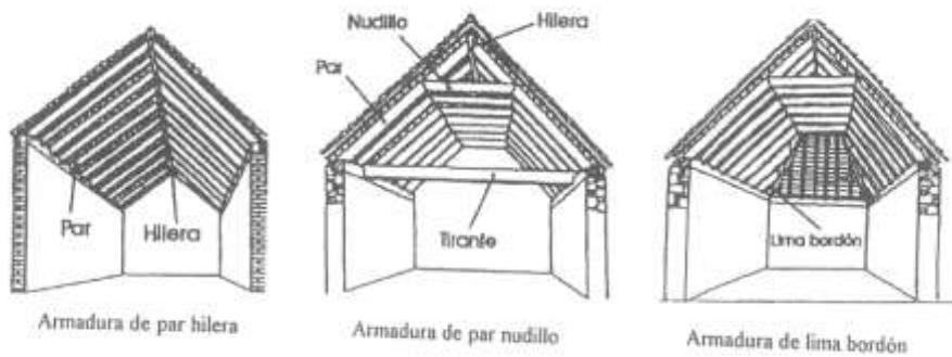
Figure 38. Drawing of ceiling types, a.Armor of couple nuckle (par hilera) b.Armor of couple row (par nudillo) c.Lima bordón. Anonymous, El Mudéjar en Andalucía Anonymous, Mudéjar en Andalucía .
