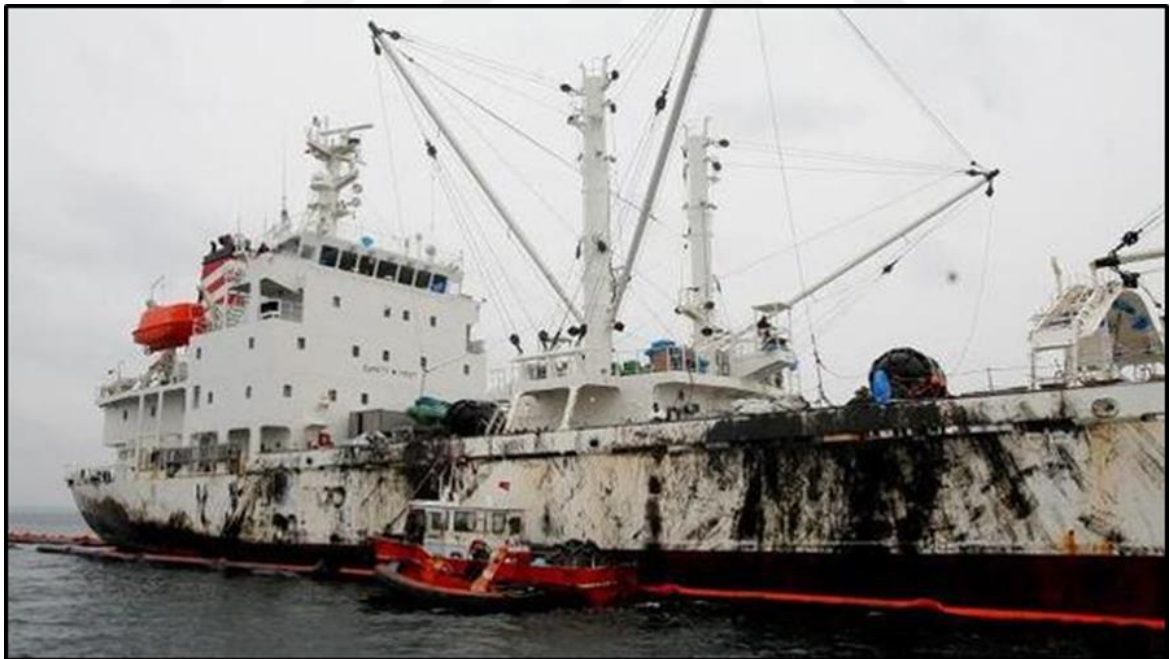
Figure 7.14. The Containment Booms were used to Control the Oil Pollution (URL-6, 2017).
