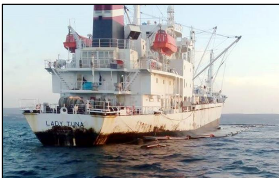
Figure 7.7. Containment of the Leaking Fuel by the Barriers (URL-4).
