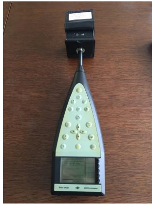
Figure 3.4. Calibration of the Sound Level Meter
