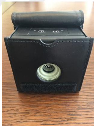
Figure 3.3. Acoustical Calibrator (Brüel & Kjaer 4231)
