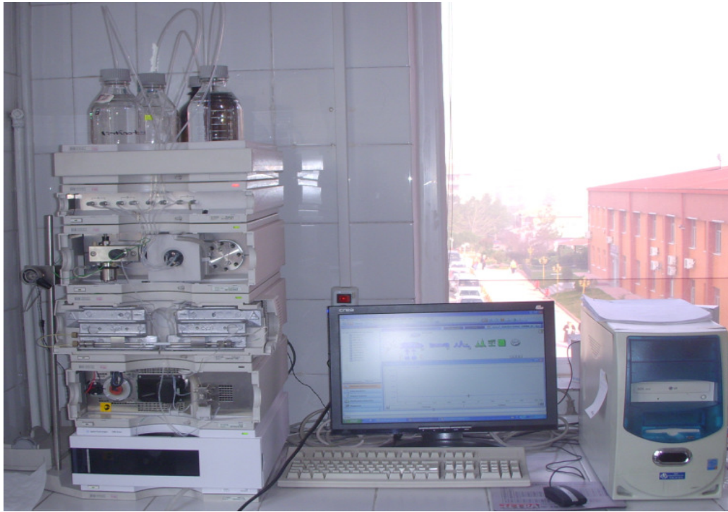
Şekil 3.2. Hewlett Packard 1100 Series-Agilent Technologies 1200 Series HPLC sistemi
