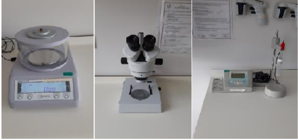
Şekil 3.4. Hassas terazi (Gibertini EOROPE 200), binoküler (HUNDZ WETZLAR), pH metre (pH ION Meter), otomatik pipet (Brand aku jet)
