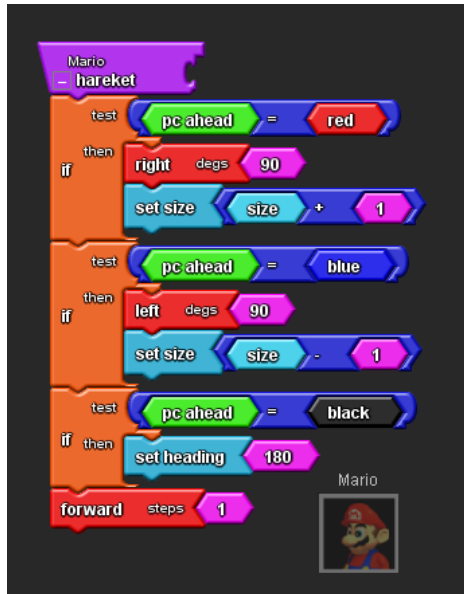
Figure 2. Procedure of movement which contains If-Else and math blocks.
