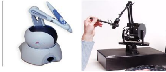
Figure 3 - Sensable Omni and Phantom 6-DOF Haptic Devices
