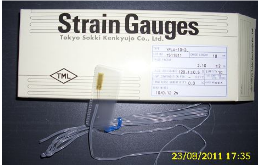
Resim 5.2.1. YFLA-10-2L Strain Gauge
