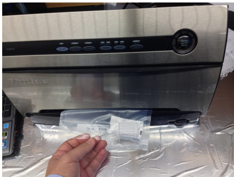
Figure 7.8 Vacuum sealer, vacuuming and sealing a bag with a chip and a bag of drying agent.
