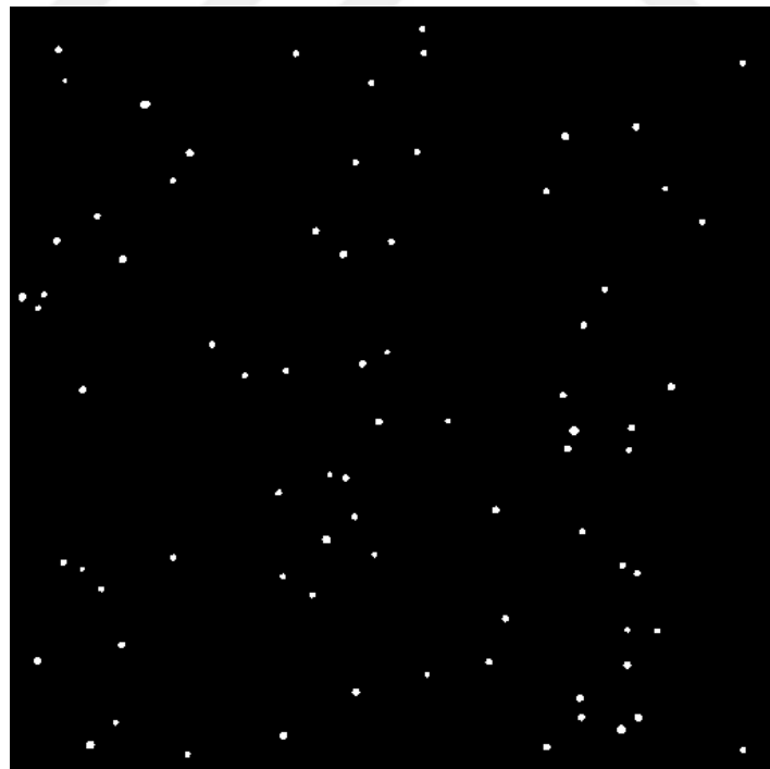
Figure 6.45 Thresholding output of cross correlation white objects indicate the cells. The image is a binary image.
