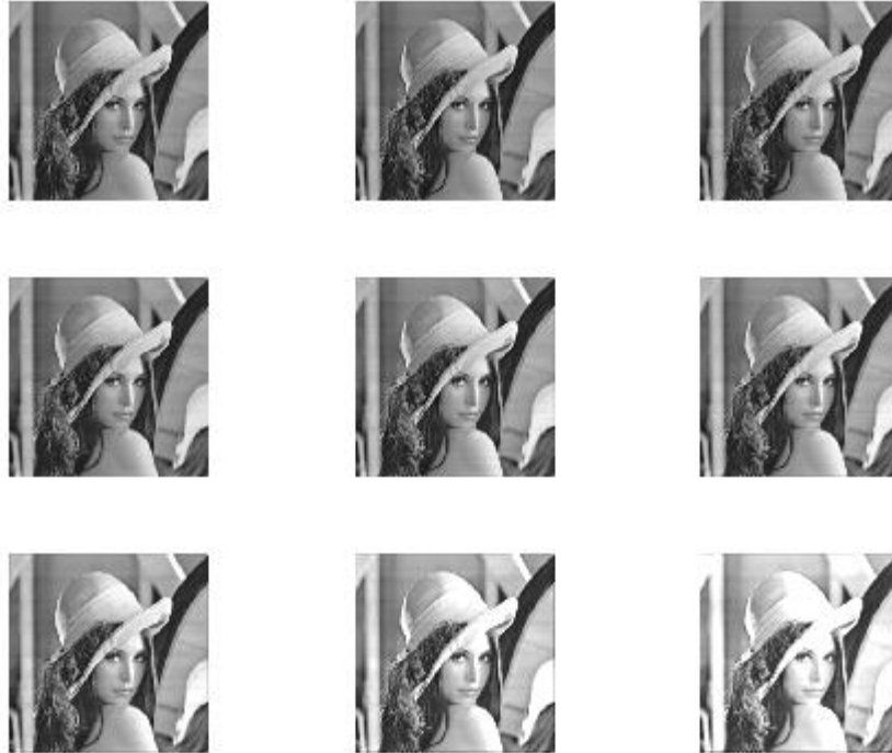
Restored images corresponding to noisy Lena images in previous figure using 2D-LMS ( \mu = 0.001 )
