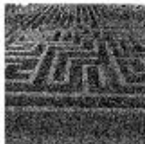
Maze Image corrupted by AWGN with different variance values and zero mean
