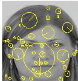
Figure 2.5. SIFT keypoints detected in a face image.
