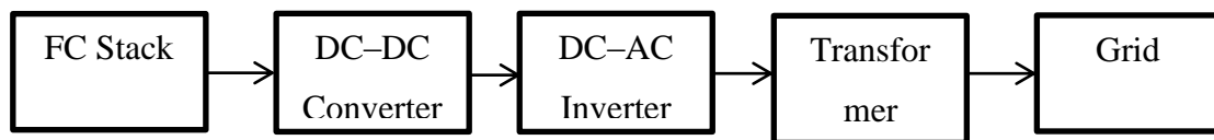
Figure 5.1 : Grid Connected Fuel Cell System
