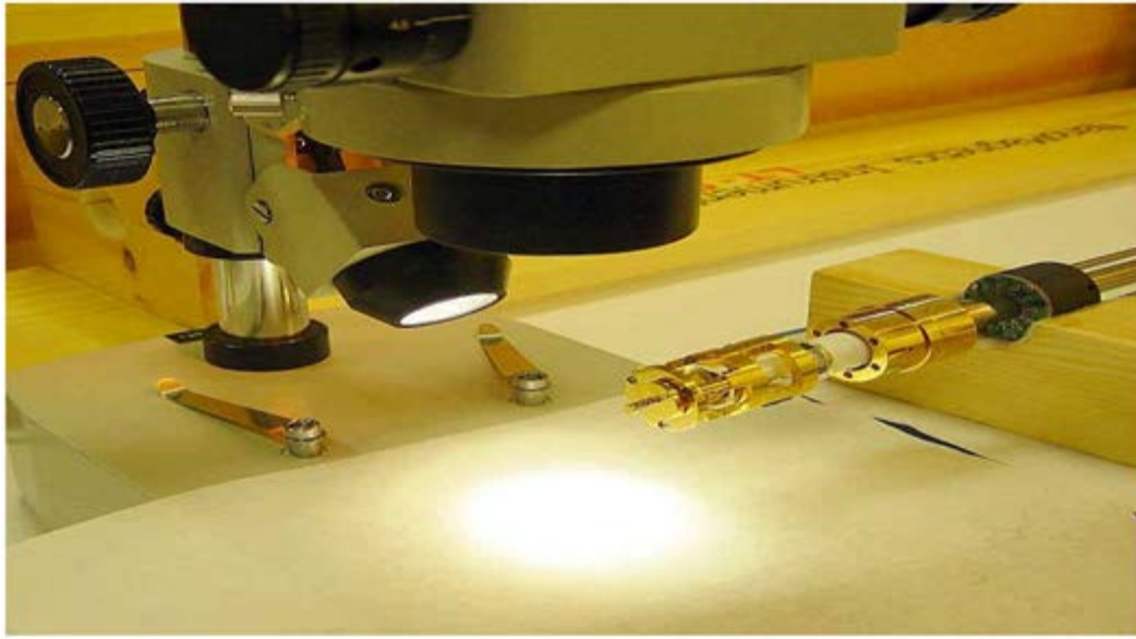
Fig.4.4 Observing the Hall probe-sample surface angle with a microscope Courtesy of Nanomagnetic instruments inc. ( http://web.nanomagnetic-inst.com ) [33].
