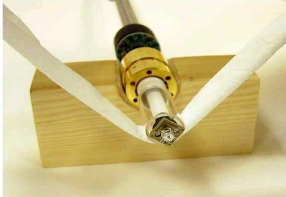
Fig.5.15 Quartz slider tube cleaning Courtesy of Nanomagnetic instruments inc. ( http://web.nanomagnetics-inst.com ) [33].
