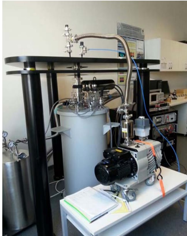
Fig.5.21 Nanomagnetic inc.LT-SHPM 1.5-320 K cryomagnetics inc. 9 tesla dry cryostat Courtesy of Nanomagnetic instruments inc. ( http://web.nanomagnetics-inst.com ) [33].
