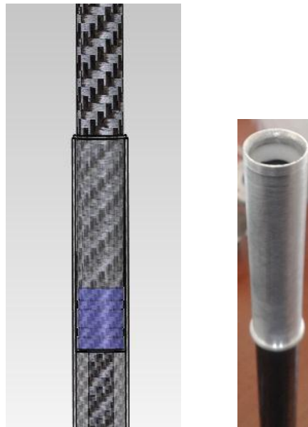
Figure 6.21: Sample rod guiding and extension mounting.
