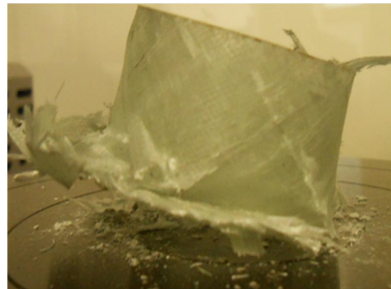
(b) Final crushed shape of glass/epoxy
