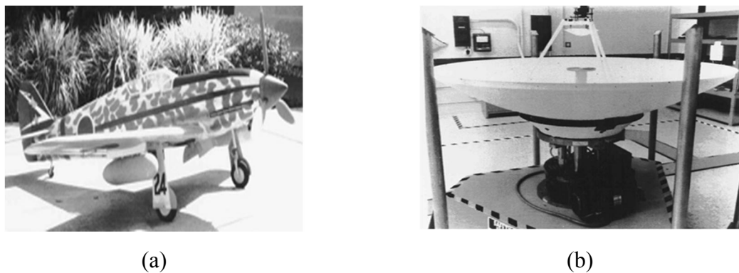
Figure 1.3 (a) German fighter plane using glass/epoxy molded fuselage and wing spars of graphite/epoxy (courtesy of Russell A. Lepre) (b) High gain antenna for space
