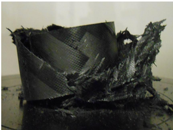
(a) Final crushed shape of carbon/epoxy
