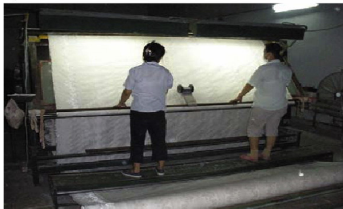
Figure 1.1 Manual inspection methods
