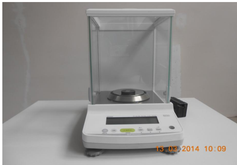
Figure 2.4: Weight scale with a sensitivity of 0.0001 grams
