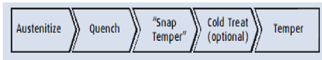
Figure 1.14: Heat treatment sequence for maximum transformation of austenite to martensite [57].
