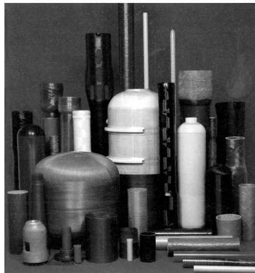
Fig 1.15 Some filament wound parts [8].
