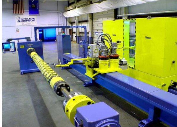
Fig 1.14 A filament winding process.
