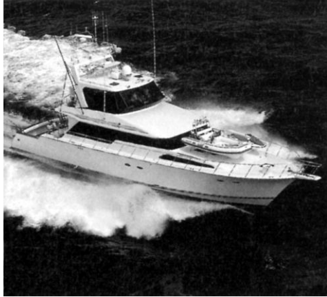
Fig 1.11 A 72-ft yacht made from wet lay-up process
