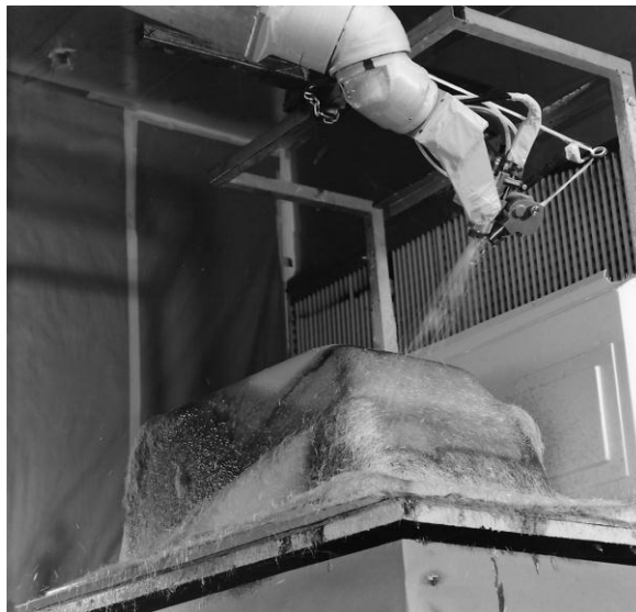
Fig 1.13 A robotic spray-up in making a bathtub [7].
