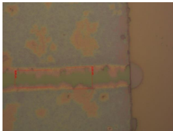
Figure 4.31: 100x microscope objective image of one of the ridges of the fabricated device (After PR removed and sample cleaned)
