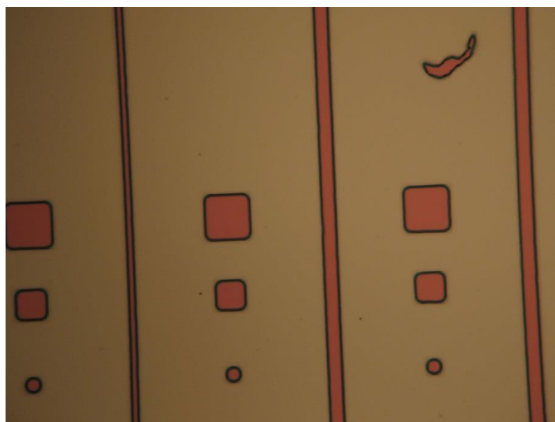
Figure 4.16: SiO 2 hard mask removed after 3-minute wet etching of Si.
