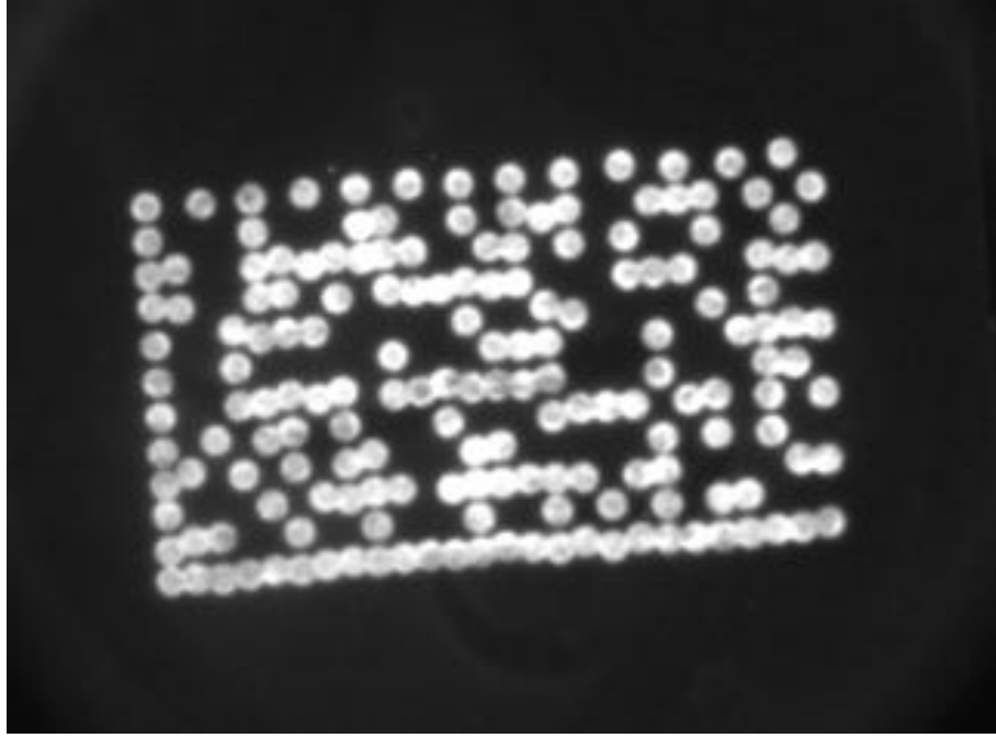
Figure 1.13 720 nm High Pass Filter Image
