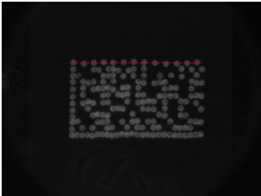
Figure 3.18 Long Frame of Timing Pattern
