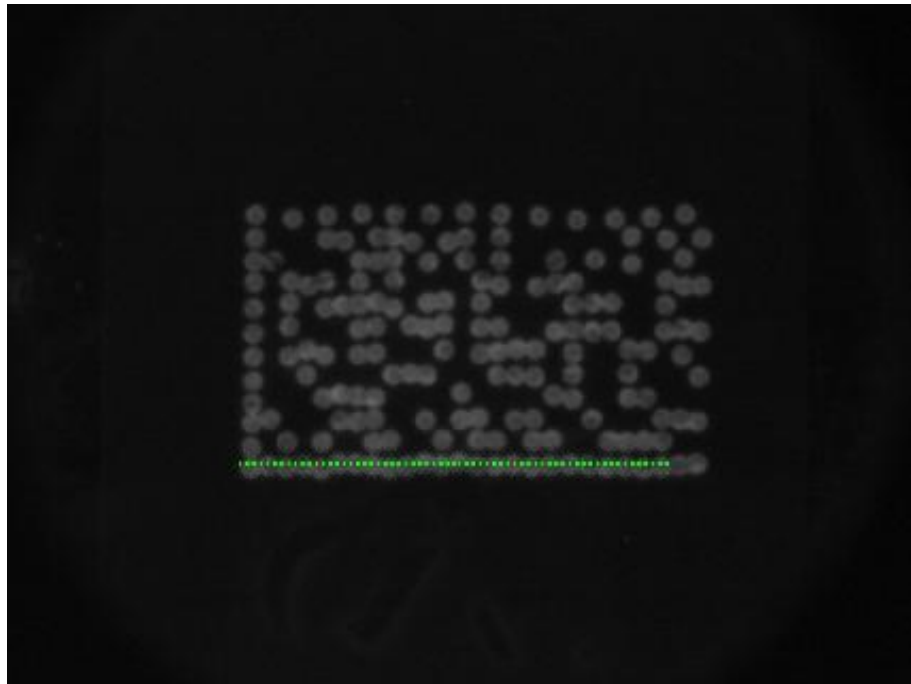
Figure 3.8 Tracing the Long Frame of the L Shape
