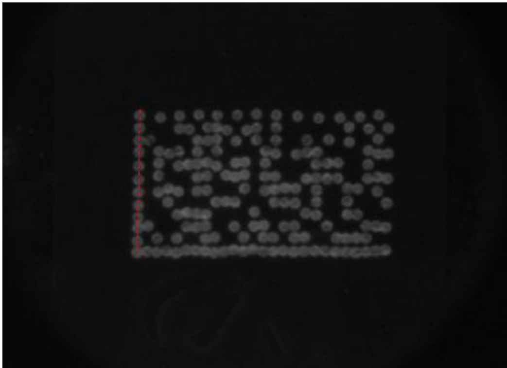
Figure 3.15 Short Frame of L Shape Finder Pattern
