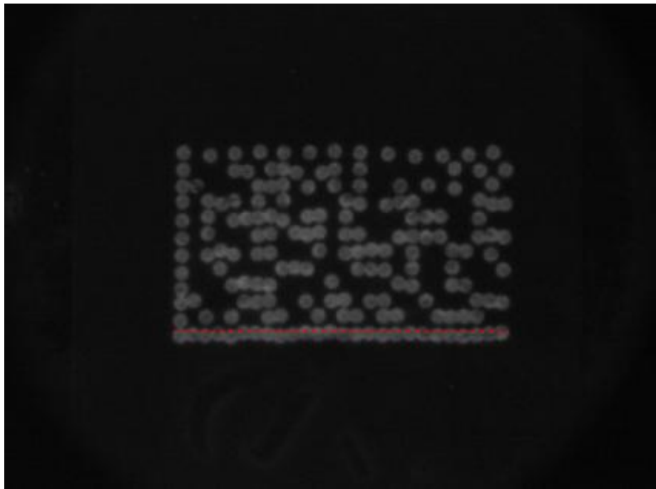
Figure 3.11. Long Frame Centers of L Shape Finder Pattern
