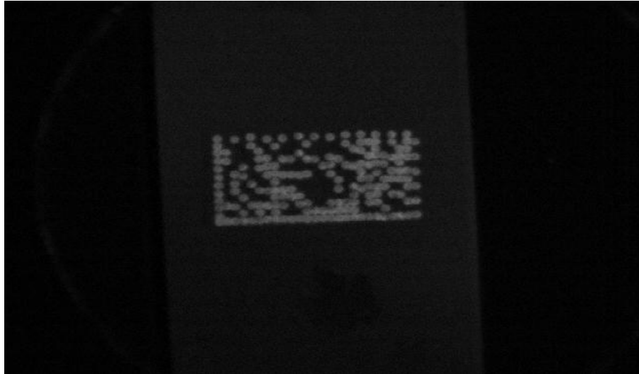
Figure 4.9: Captured Invisible 2D Data Matrix via high pass filter
