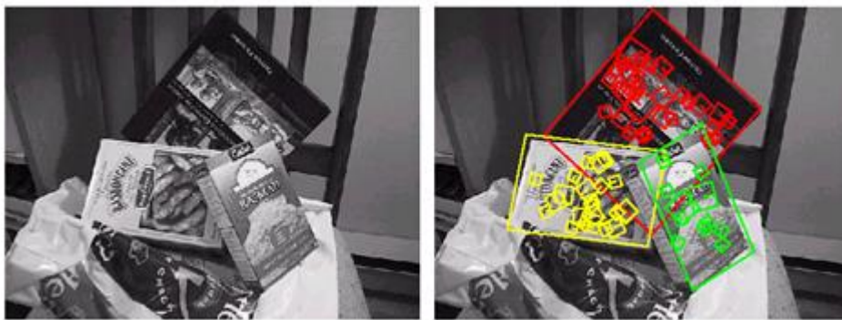
Figure 1.1 Images of objects are shown in first one. The result of object recognition is on the second image with using feature points.
