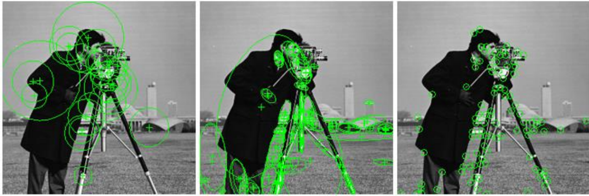
Figure 2.1. Extracted feature points in an image are shown. SURF detector on the left, blob detector on center and corner detector on the right side.
