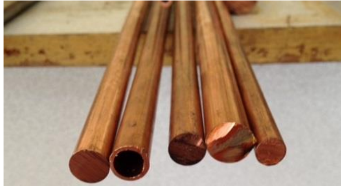
Figure 3.2.3: Cu sheath material for multicore manufacturing
