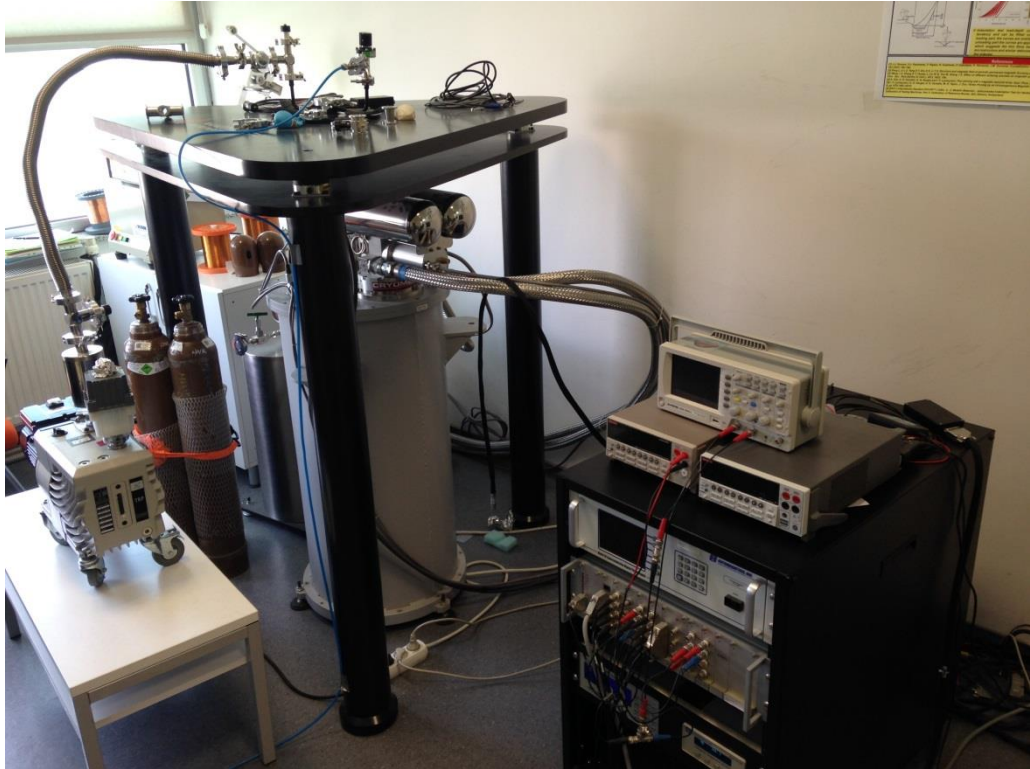
Figure 4.2.1.2: 9 Tesla Closed He Cycled Dry Cryostat System for electrical and magnetic resistivity measurements.
