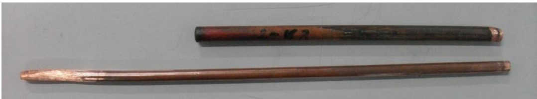
Figure 3.4.2: Cu sheath MgB_2 mono-core extended rods by made hot extrusion method.
