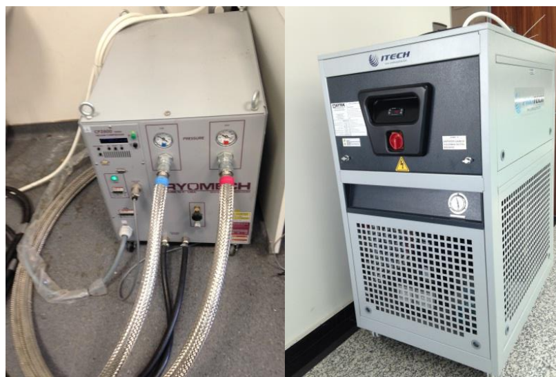
Figure 4.2.1.3: a) Helium Cooler Unit , b) Water circulation Chiller System.
