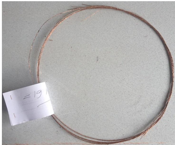
Figure 3.3.5: Single piece and 40 meters mono-core mechanical-alloyed MgB 2 powder made SC wire.
