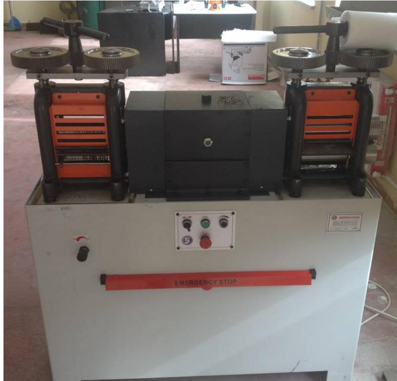
Figure 3.5.1: 30 channel specific design wire drawing machine.
