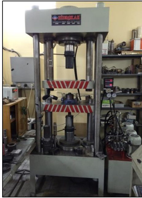
Figure 3.4.1: 150 tons of compressive force capacity hydraulic press in Erciyes Univ. Composit Lab.
