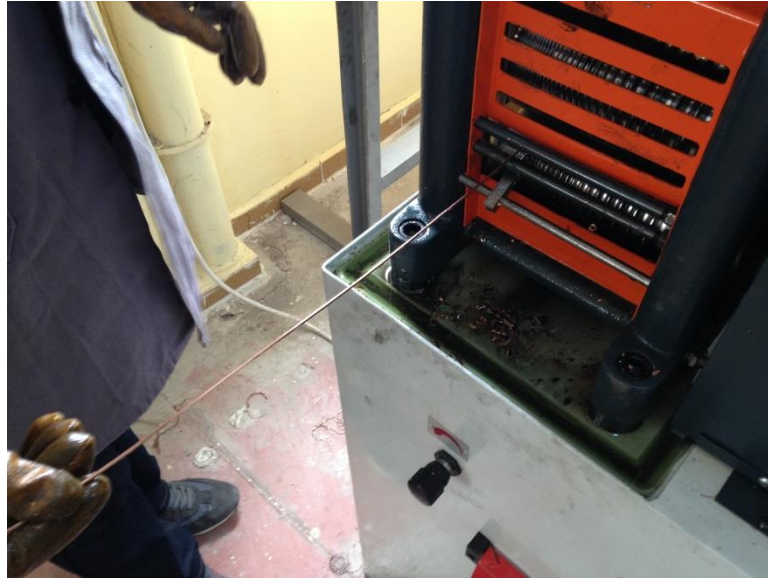
Figure 3.5.2: Wire drawing process.
