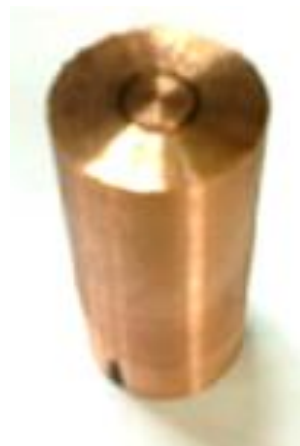
Figure 3.2.2: Cu billet by using PIT method.
