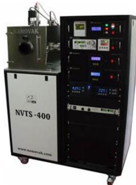
Figure 2.1. The thermal & sputter combined PVD system, NVTS-400, at the thin-films fabrication laboratory of Melikşah University.
