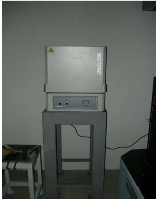
Figure 3.1 Muffle furnace which is used heat treatment processes (PLF 110/6 Protherm)
