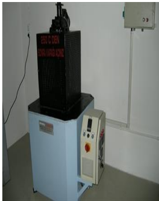
Figure 3.2 Salt bath furnace which is used austempering processes
