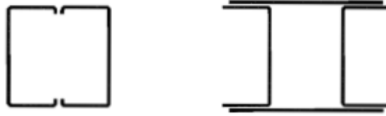
c) Closed built-up sections
