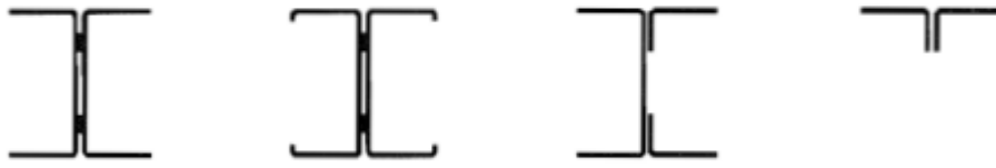
b) Open built-up sections
