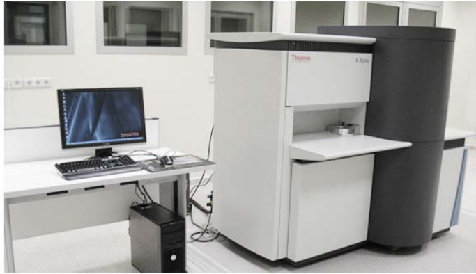
Şekil 9: XPS cihazı (Thermo, K-Alpha - Monochromated high-performance XPS spectrometer)
