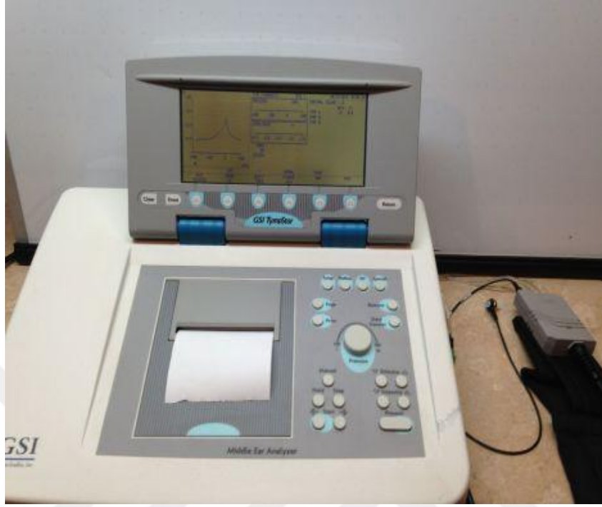
Şekil5: GSI (Grason-Stadler Inc.) Tympstar Middle Ear Analyzer Version 2
