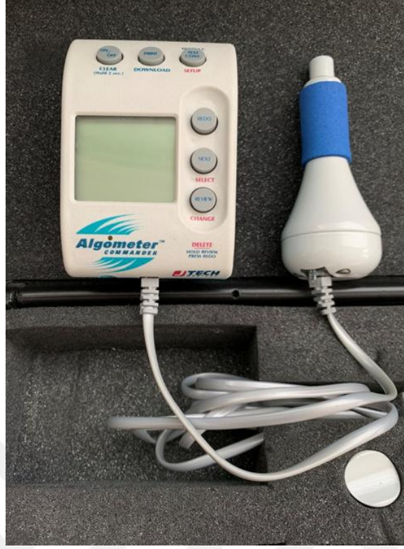
Şekil 3.1 Algometre (Algometer Commander JTECH™ Salt Lake UT)
