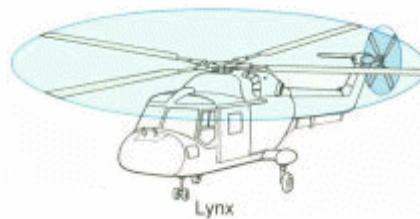
Figure 2.1: Single Rotor Configuration [7]
