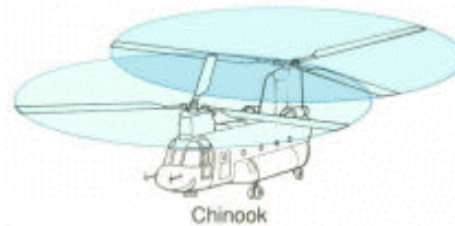
Figure 2.3: Tandem (fore and aft) Rotors [7]
