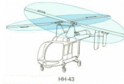
Figure 2.5: Two Intermeshing Rotors [7]
