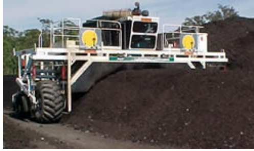
Figure 2.1 : Mixing operation of turned windrow.
