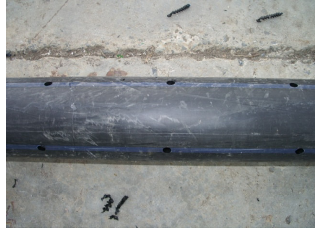
Figure 3.2 : Aeration system used in aerated static pile.
