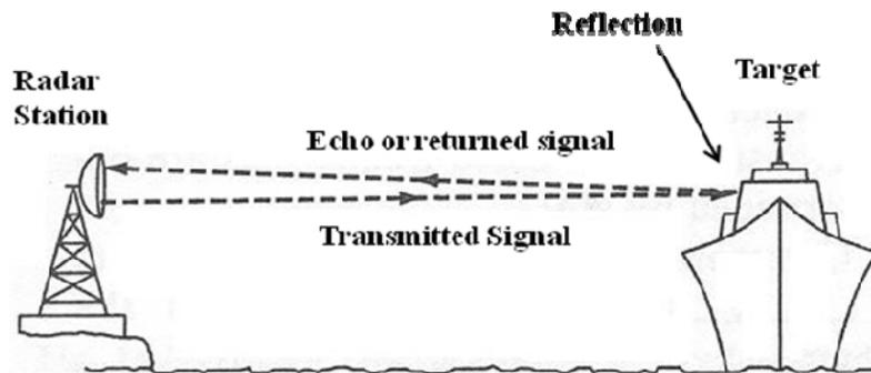
**Figure 2.1 :** The elementary concept of radar [8].
