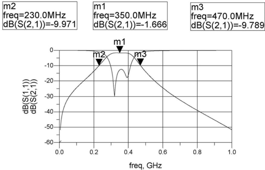
**Figure 3.15 :** Frequency response of the pre-selector filter.
