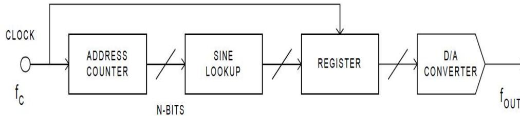
**Figure 3.1 :** Fundamental direct digital synthesis system.
