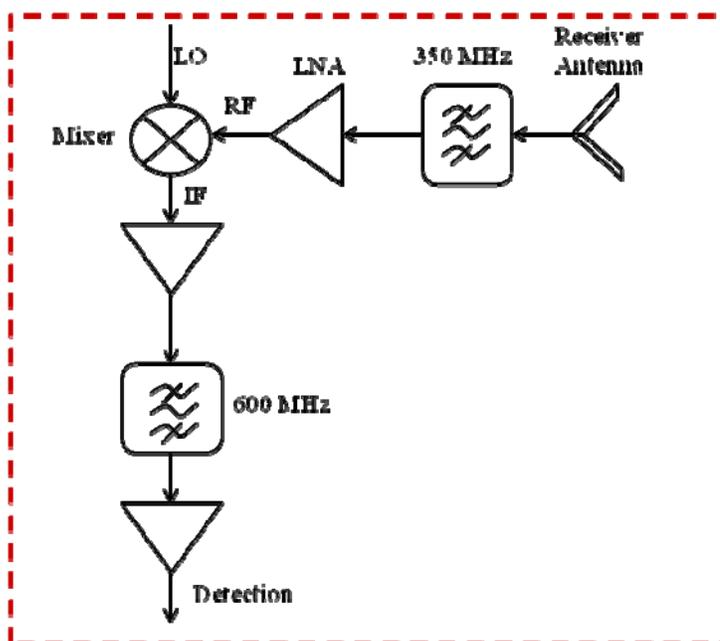
**Figure 3.14 :** The receiver architecture.
