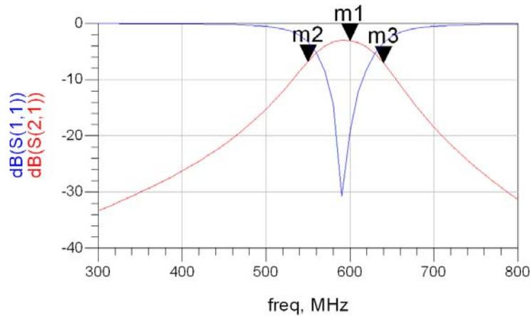
Figure 3.23 : Frequency response of the filter.
