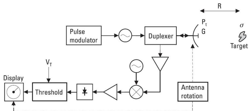
**Figure 2.6 :** Block diagram of pulse radar [7]
