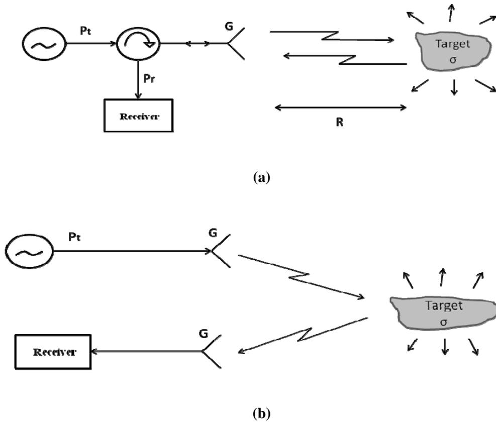
**Figure 2.2 :** Basic monostatic and bistatic radar systems. **(a)** Monostatic radar system. **(b)** Bistatic radar system [4].
