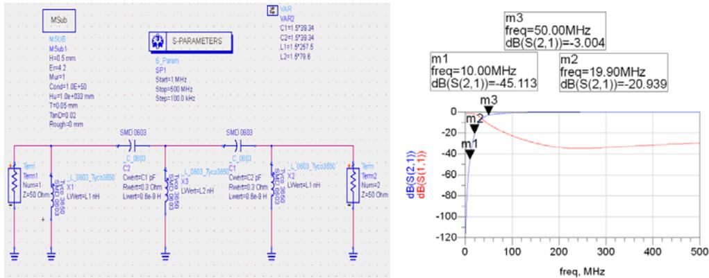
**Figure 3.11** : ADS application page and frequency response of the filter.
