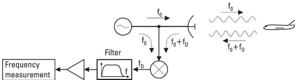
**Figure 2.7 :** Basic doppler radar [7].
