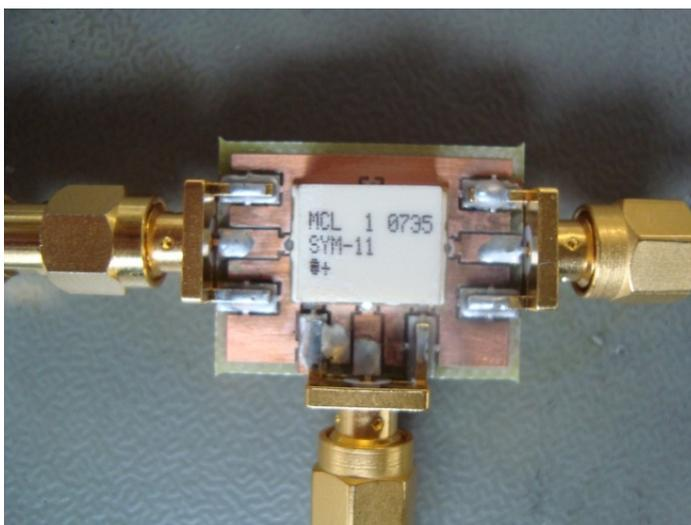
**Figure 3.21** : SYM-11 double-balanced frequency mixer.
