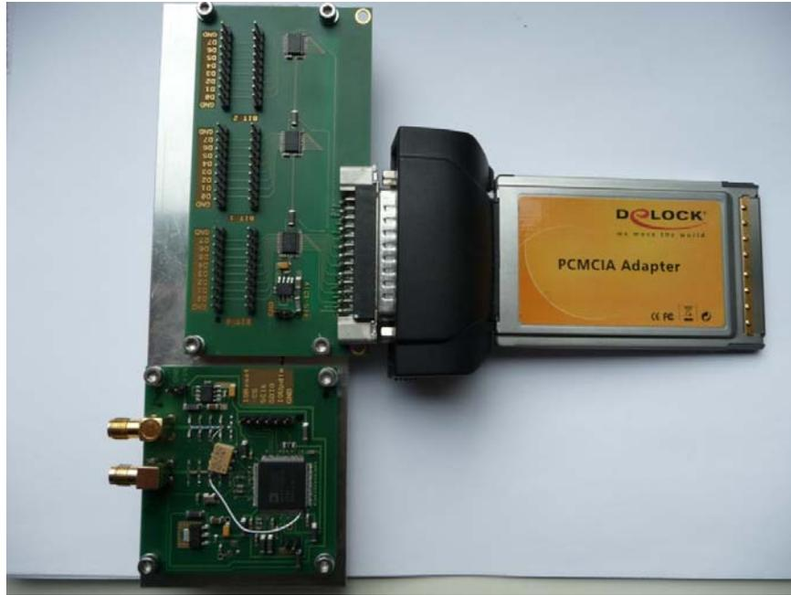
**Figure 3.5 :** AD9910 application board.
