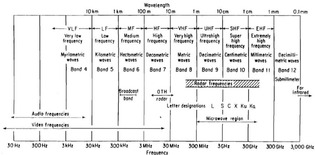
Figure 2.5 : Radar frequency and electromagnetic spectrum [5].
