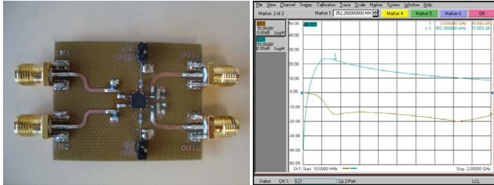
**Figure 3.19 :** HMC816 application board and its network analyzer response.
