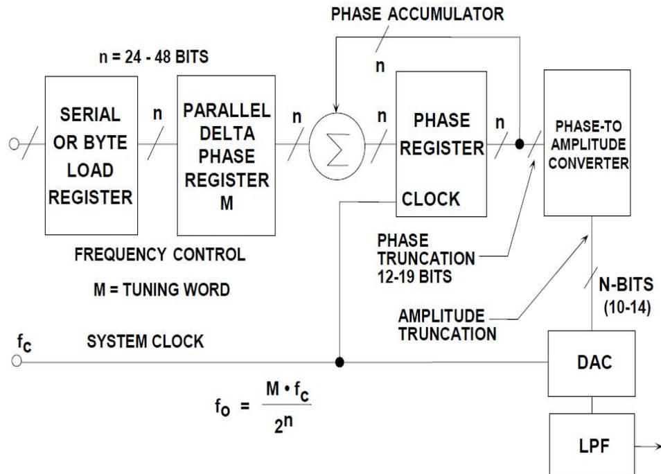
**Figure 3.2 :** A flexible DDS system
