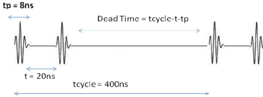
**Figure 3.7 :** The basic concept of the pulse train [14].
