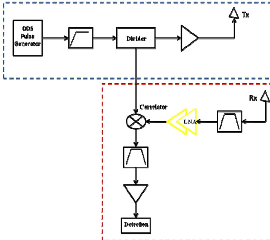
**Figure 1.1** : The transceiver architecture of the pulse radar system.
