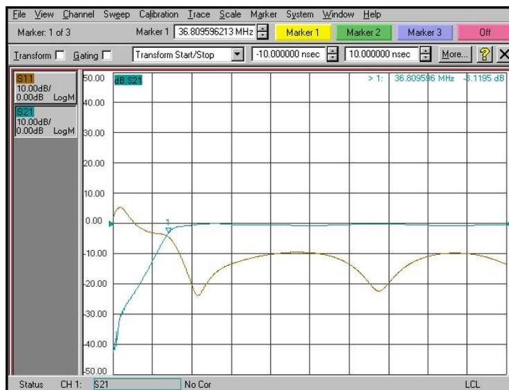
**Figure 3.12** : The network analyzer response of 50MHz filter.
