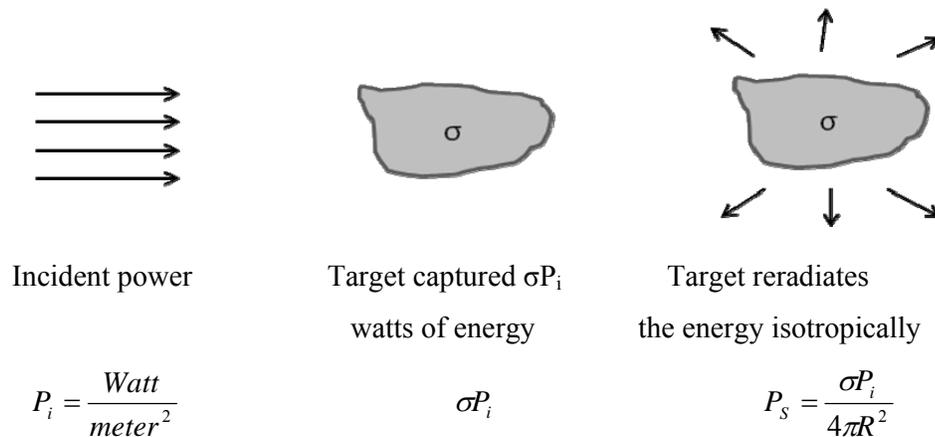
**Figure 2.3 :** Intuitive definition of radar cross section.
