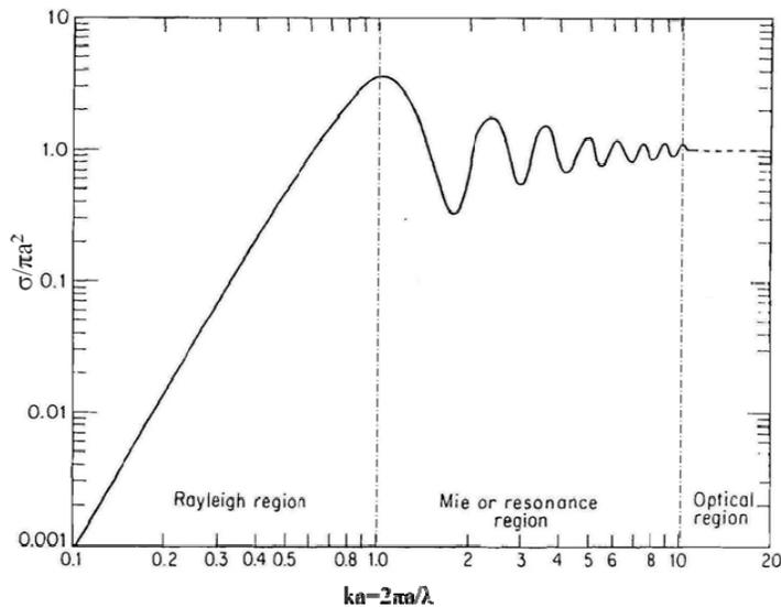
**Figure 2.4** : Radar cross section of a perfectly conducting sphere.
