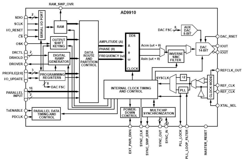
**Figure 3.4 :** Detailed block diagram of AD9910.
