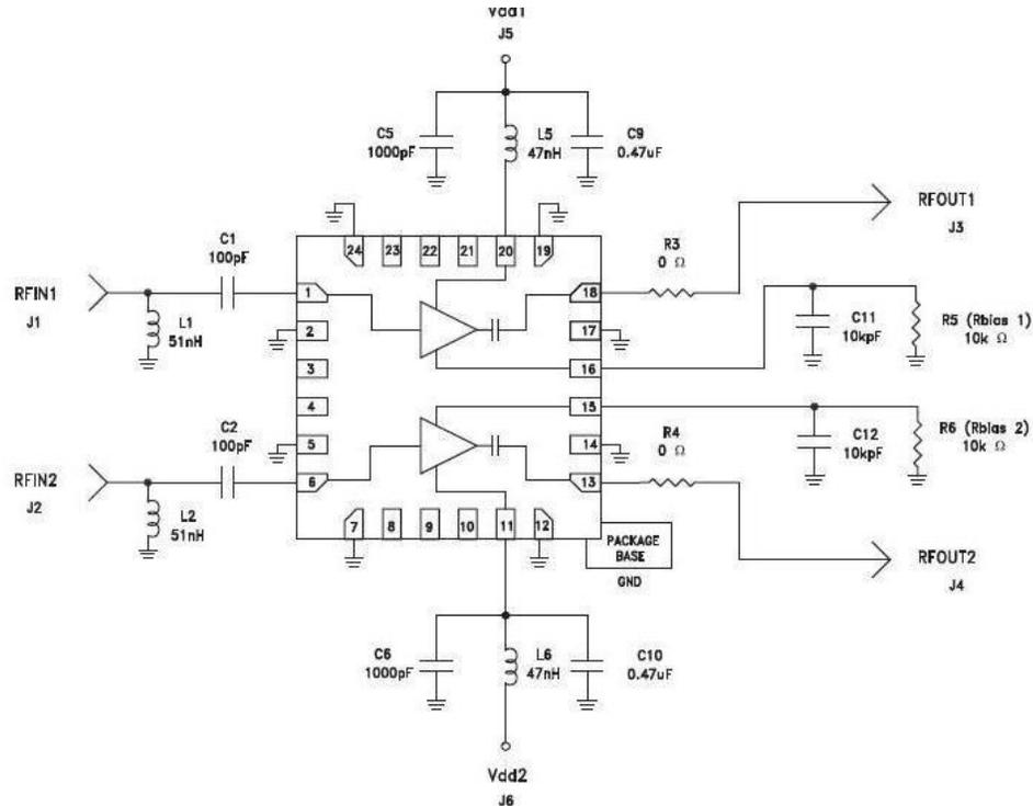
**Figure 3.16 :** Application Board of HMC816.
