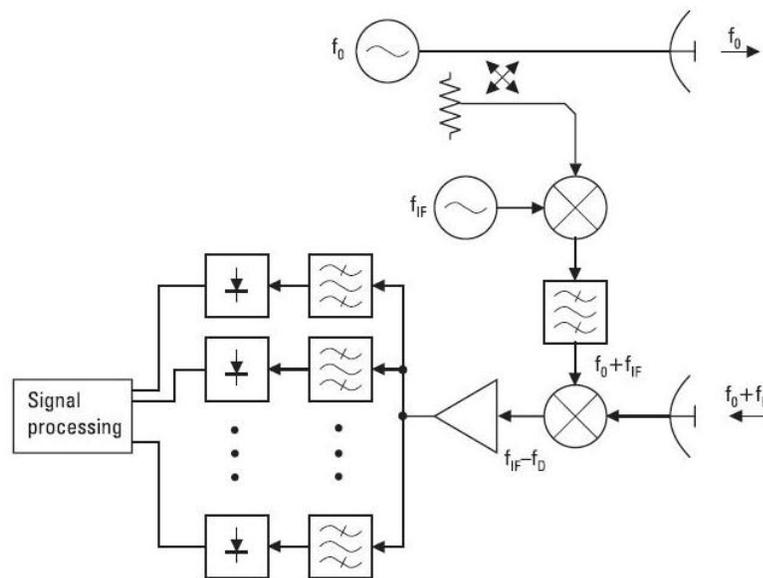
**Figure 2.8** : Doppler radar having separate antennas for detection [7].
