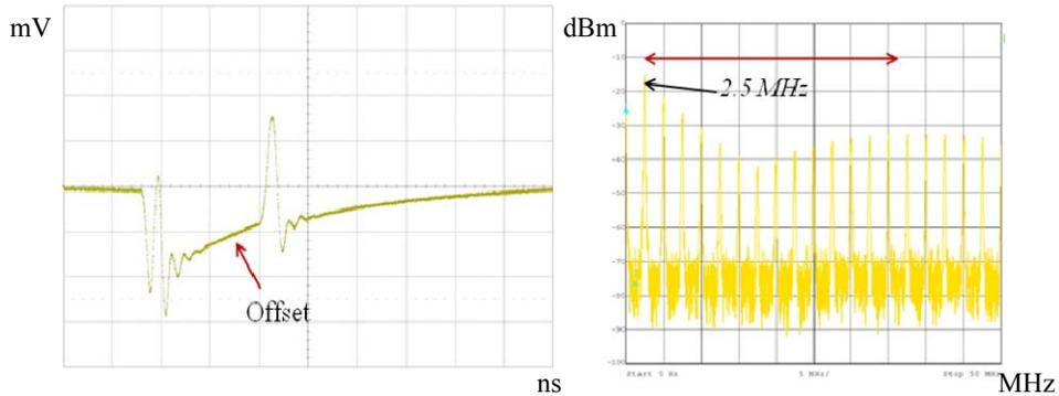
**Figure 3.10** : DDS Output offset representation in time and frequency region.
