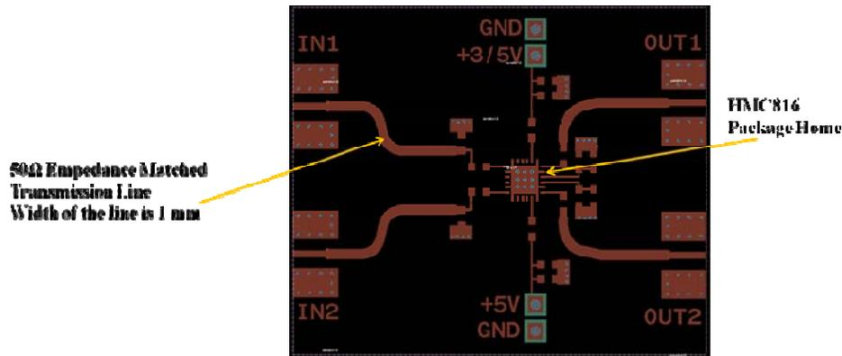
**Figure 3.17 :** ADS Layout of HMC816.
