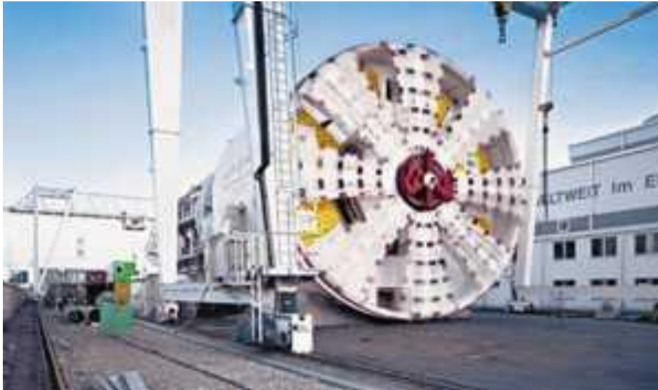
Figure 2.8 : An example of mixshield with open type cutterhead [3].
