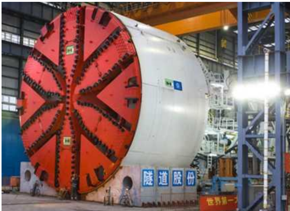
Figure 2.9 : Mixshield with closed type cutterhead [3].
