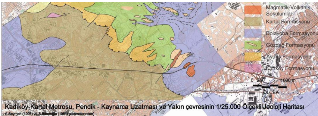
Figure 3.7 : Geological map of the tunnel route [10].
