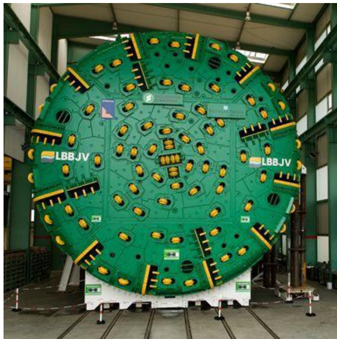
Figure 2.6 : Double shield machine for Brisbane Australia with a diameter of 12.4 m [3].
