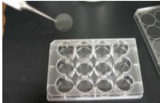
Figure 2.10 : Glass coverslides on which calcium phosphate layers were formed following the mineralization reactions.
