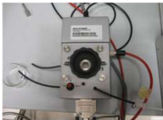
Figure 2.8 : Server-client architecture. The QCM flow cell, through which initially the buffer to clean the system, and then the tested sample solution at increasing concentration are channeled.
