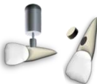
Figure 2.9 : Schematic description of the procedure for cutting cylindrical specimens from the root.
