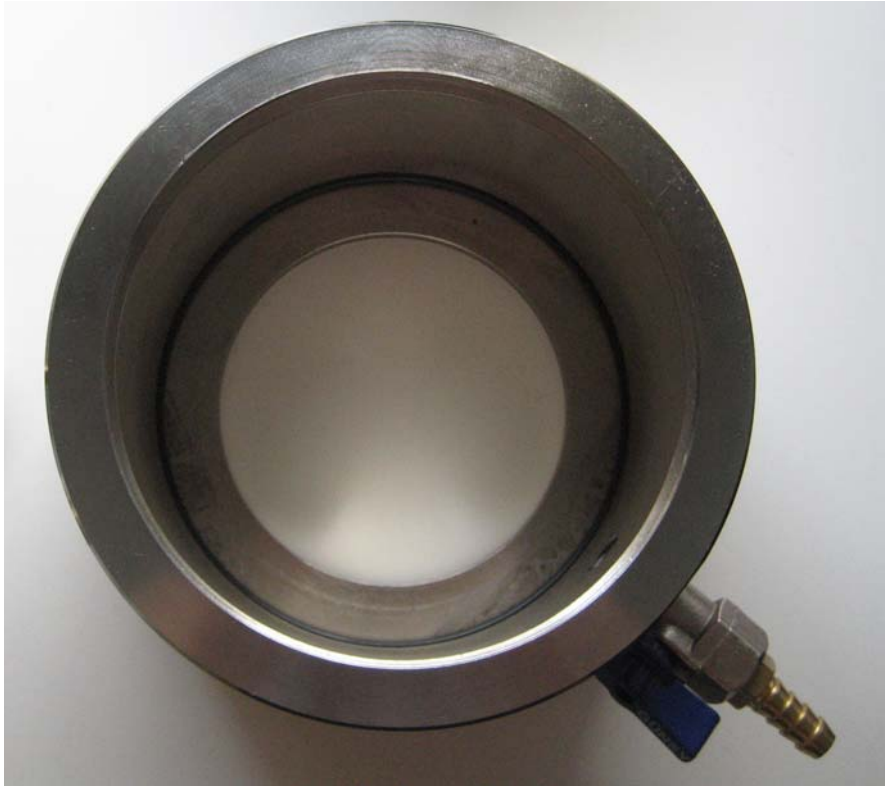
Figure 3.6: Back Pressure Cell
