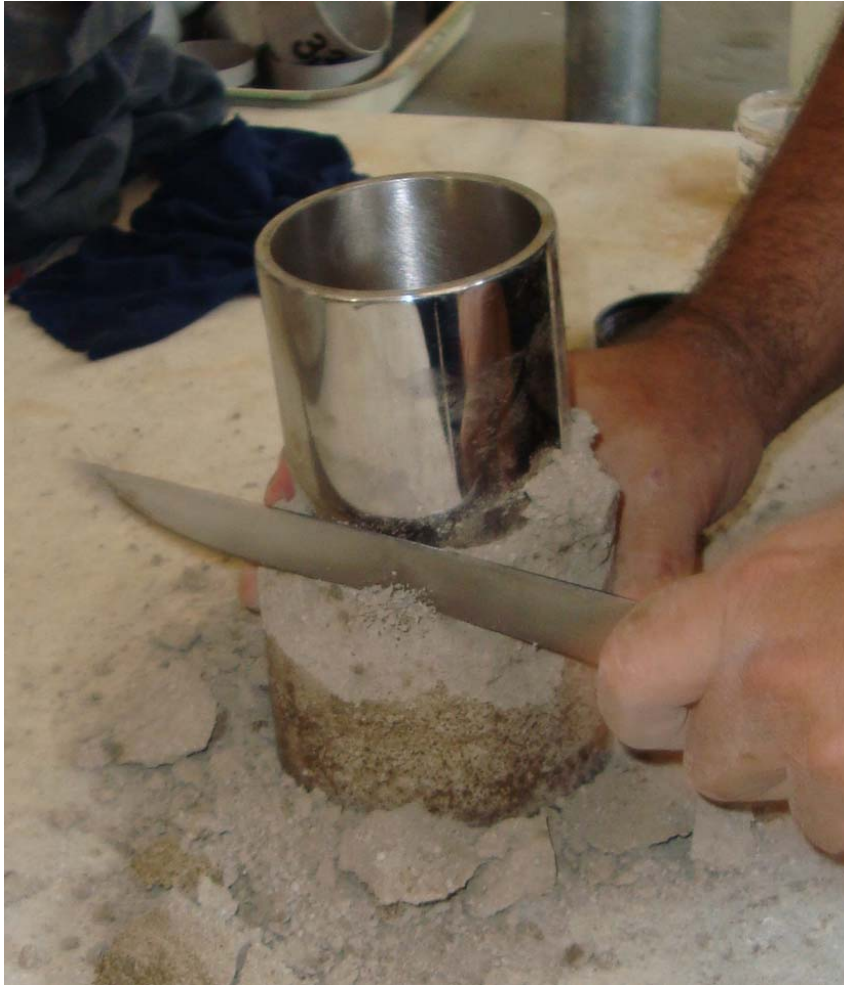
Figure 3.17: A Photograph Taken During the Penetration of the Sampler into the Specimen
