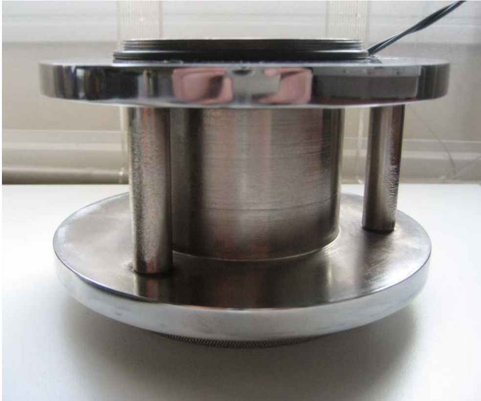
Figure 3.5: The ring body, top and bottom collars and the pivot bolts
