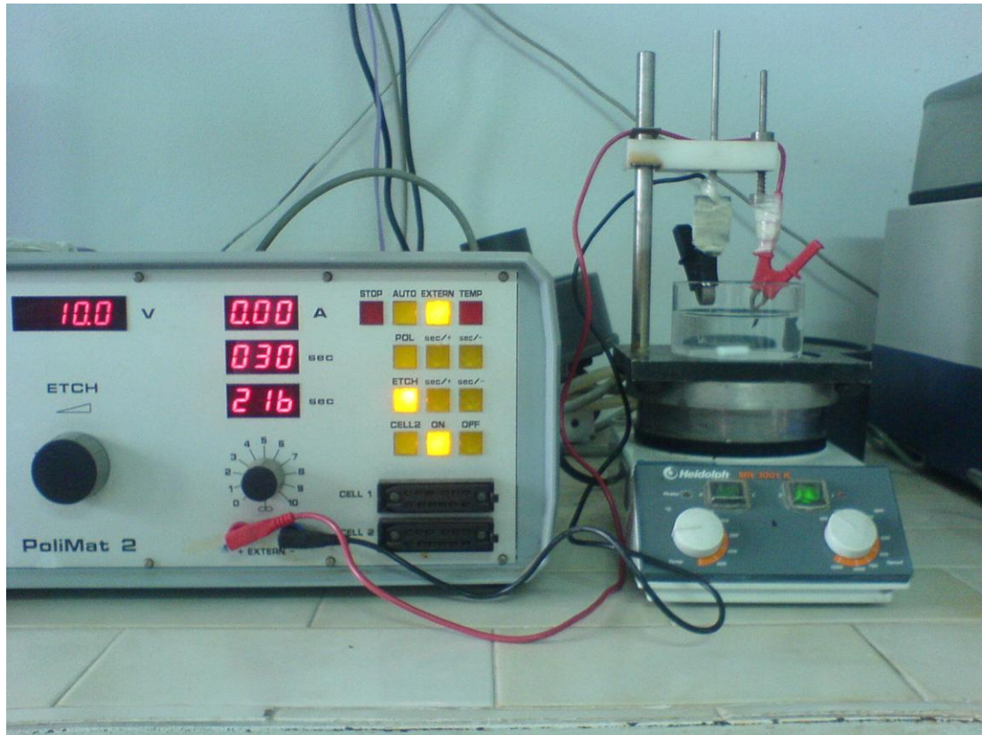
Figure 6.2: Anodic oxidation equipment used in this study.
