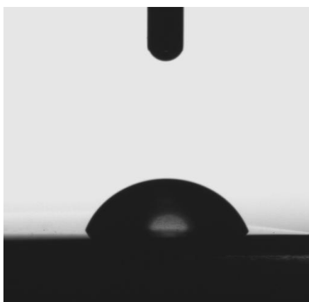
Figure 7.12: View of a water droplet 10s after dropped on CP titanium sample anodized at 10V for 10 minutes
