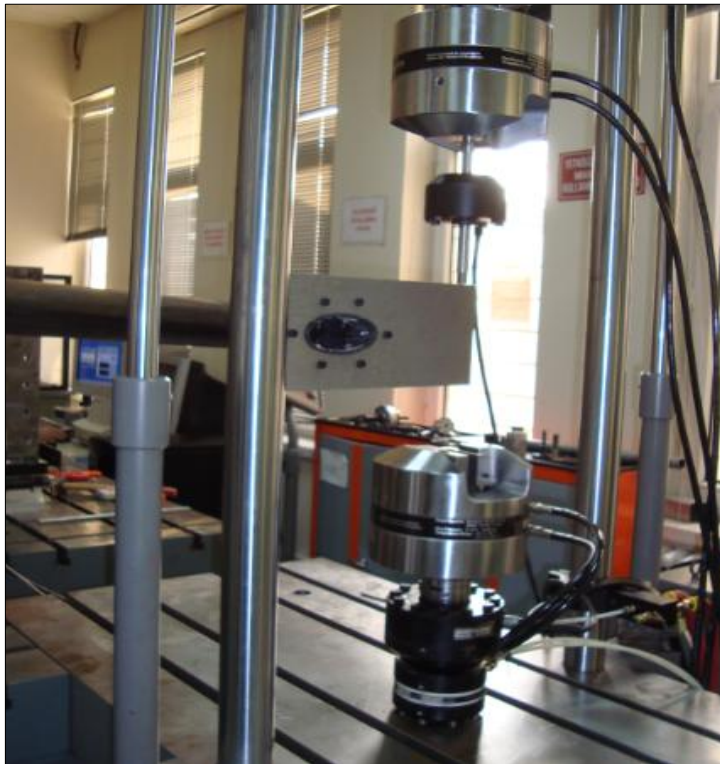
Figure 5.3: Torsional-bending test mechanism.
