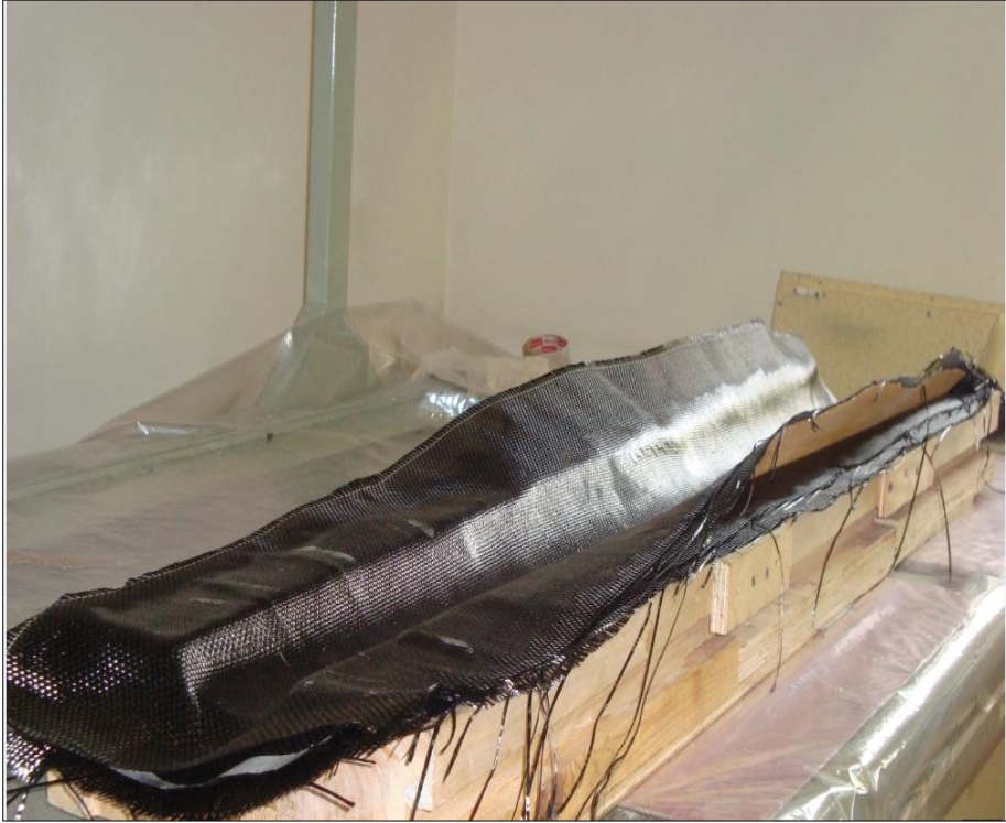
Figure 4.9: Hand lay-up technique.
