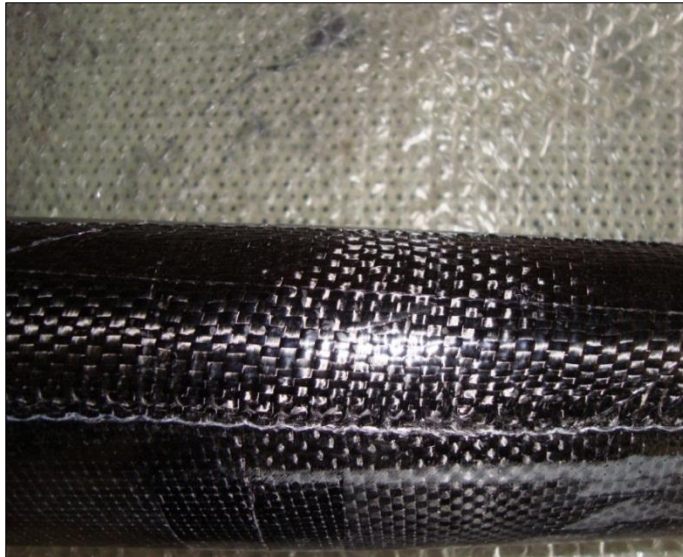
Figure 4. 15: Outside tape band after cured.
