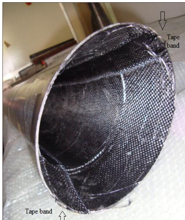
Figure 4.14: Inside the tape band after cured.
