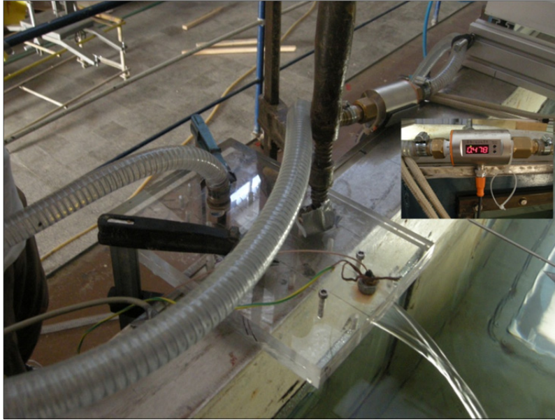
Figure 4.8 : Flush mounted hot film probe calibrator.
