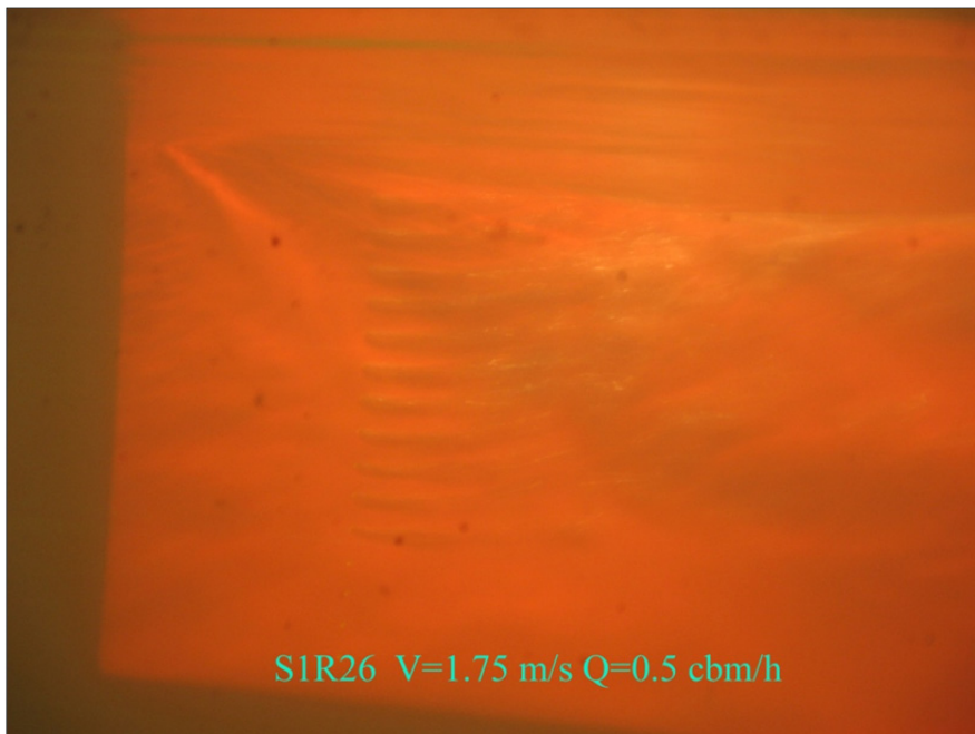
Figure 3.4 : Vertical flat plate test for V=1.75 m/s and Q=0.5 m 3 /h.
