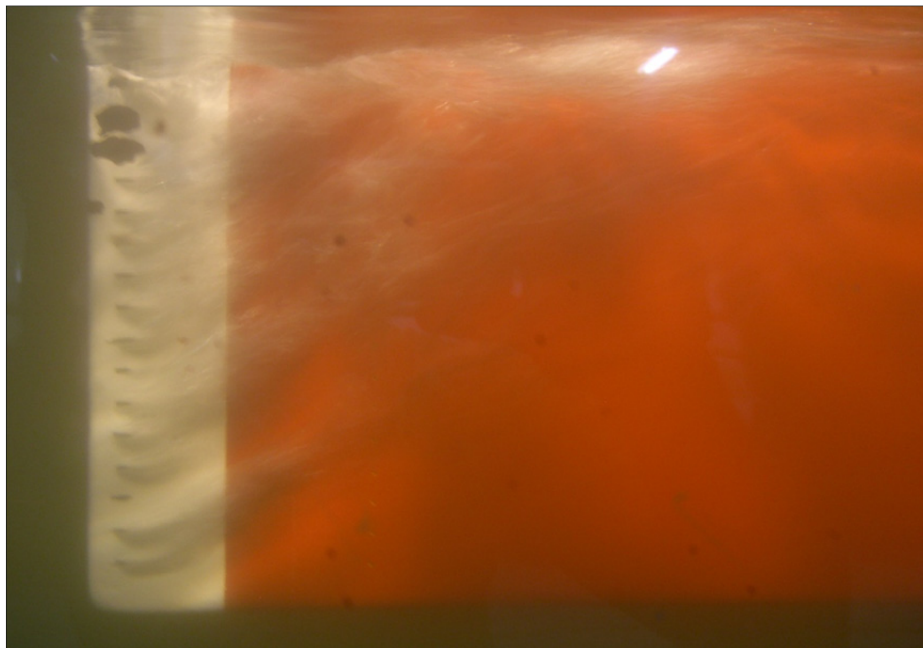
Figure 3.8 : Vertical flat plate experiment (air was injected from leading edge)
