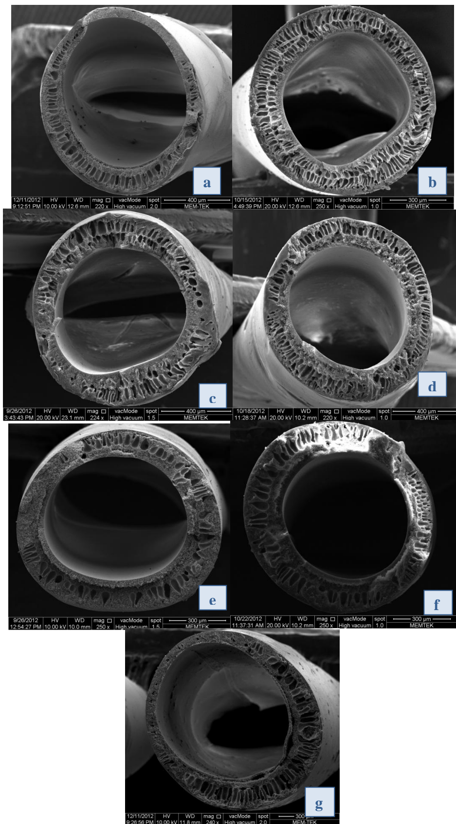
Figure A.4 : Cross sectional view of #1 membranes without post treatment. a) Pristine 1, b) 0.2COOH 1, c) 0.4COOH 1, d) 0.8COOH 1, e) 0.2OH 1, f) 0.4OH 1, g) 0.8OH 1.
