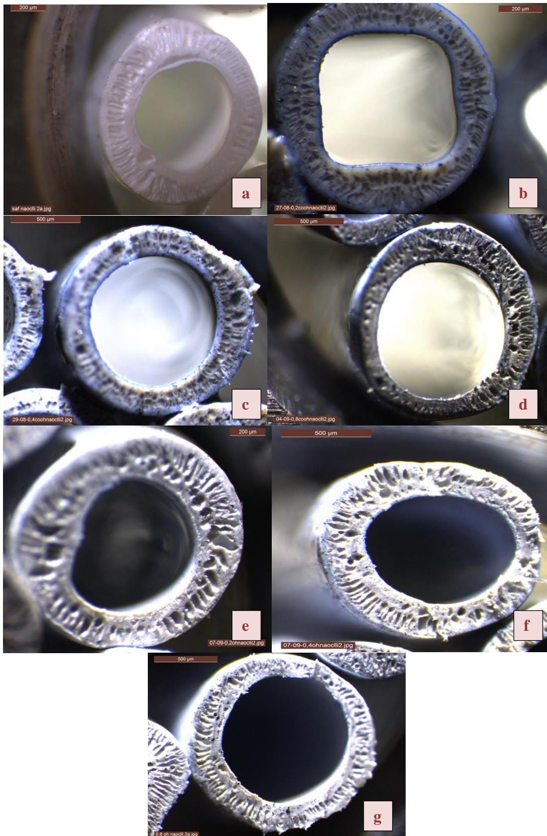
Figure 4.3 : Cross section stereo microscope pictures of #2 membranes. a) pristine 2, b) 0.2COOH 2, c) 0.4COOH 2, d) 0.8COOH 2, e) 0.2OH 2, f) 0.4OH 2, g) 0.8OH 2.
