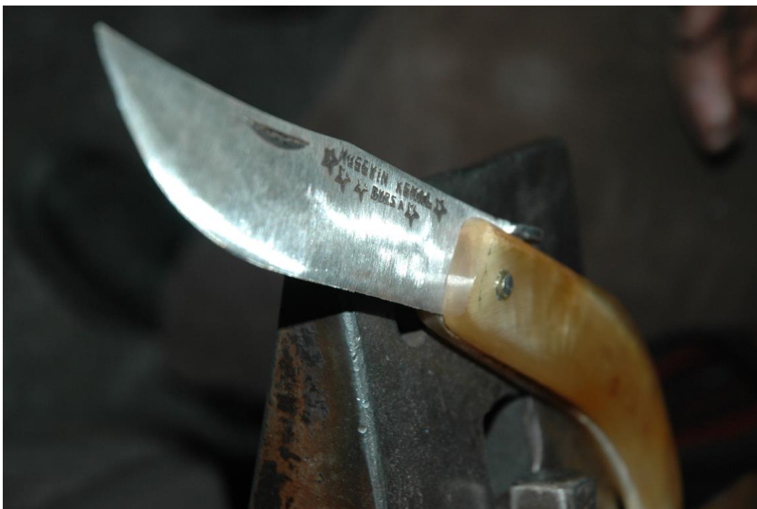
Figure 4.4: A ‘five-star’ knife by Altıparmakogulları. Instead of milimetric dimensions which would potentially be confusing for the customers, cutlers use stars as indicators of size.
