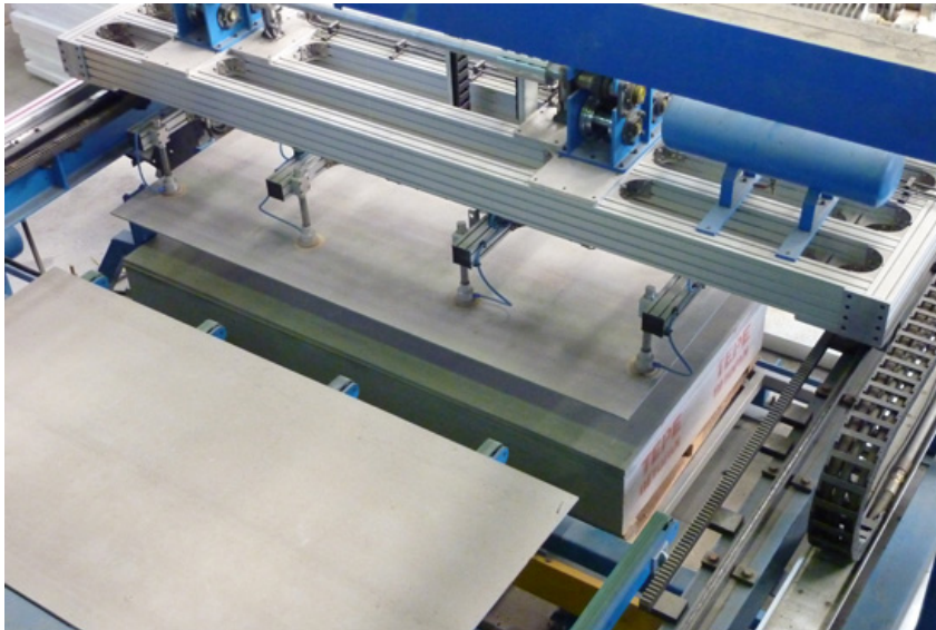
Figure 3.3 : Sandwich panel manufacturing machine (Url-10).
