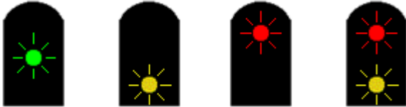
Figure 2.53 : Flashing dwarf signal aspects [21].
