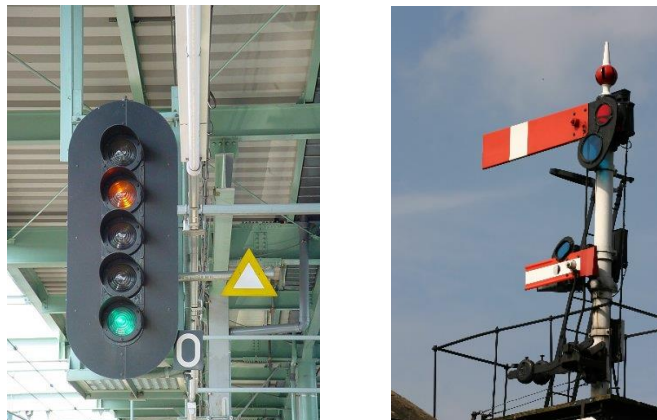
Figure 2.9 : Sample Railway Signals. Left: Light Signal, right: Semaphore Signal [13]
