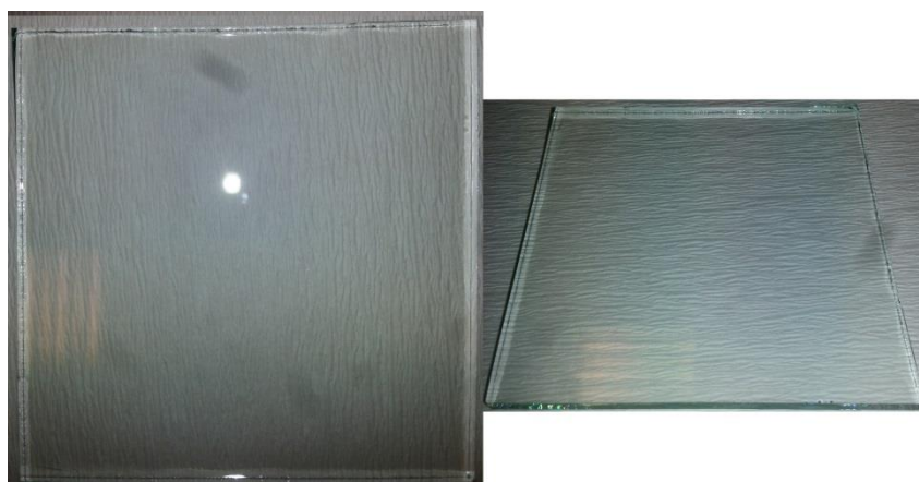
Figure 4.1: Uncoated glass substrates for the mechanical tests (8 x 8 mm plain, thickness: 3.2 mm).
