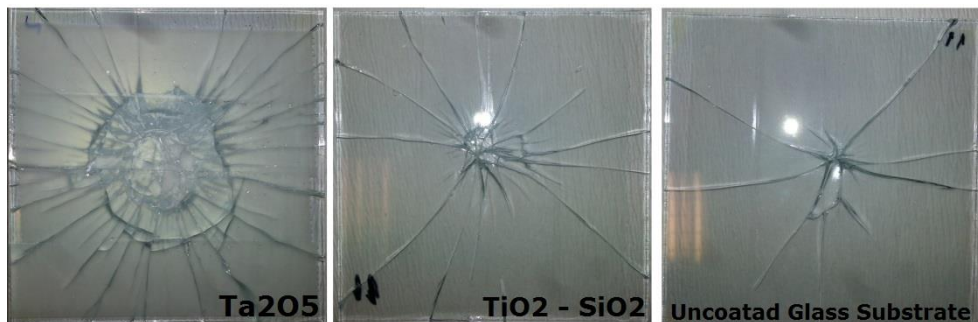
Figure 5.7: Broken glasses with different coatings and three different failure types.
