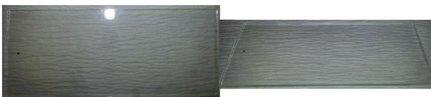
Figure 4.2: Ta 2 O 5 thin film coated Corning glass 2947 (7.62x2.54 mm plain, thickness: 1mm).
