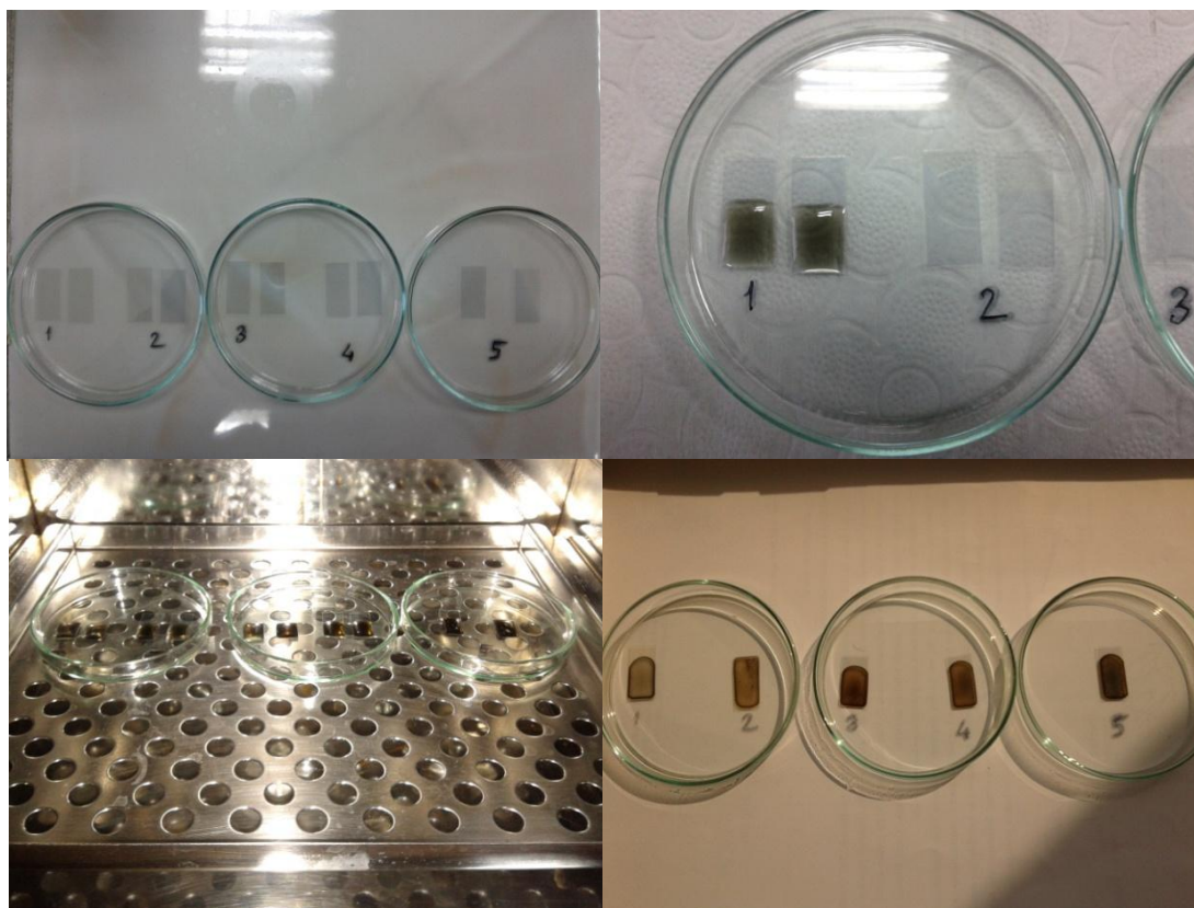
Figure 4.49 : Preparation stages of thin-films and the resultant samples.
