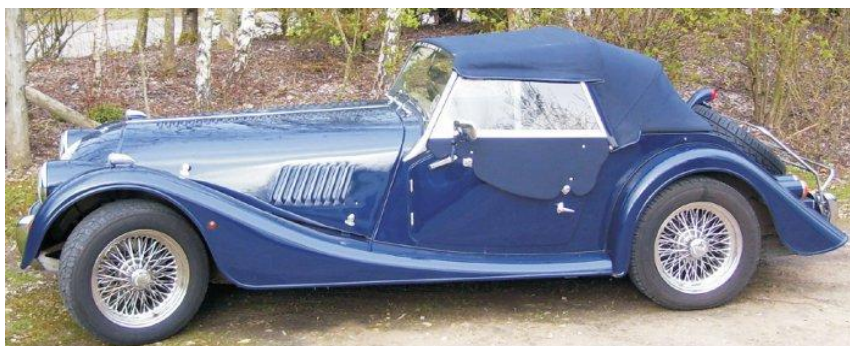
Figure 2.29 : The soft tops for high quality cars are produced from almost pure homopolymer of PAN.
