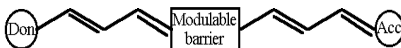
Figure 2.44 : Insertion of a “spacer” to separate the donor and acceptor (functionalized chain ends).
