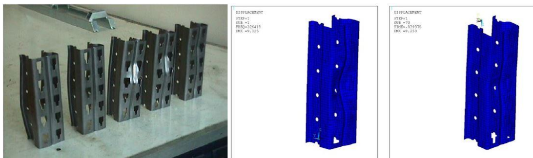
Figure 2.24 : Experimental collapsed specimens and deformed shapes from FE analysis [58].
