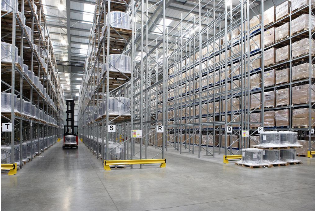
Figure 1.14 : Pallet racking structure example [15].
