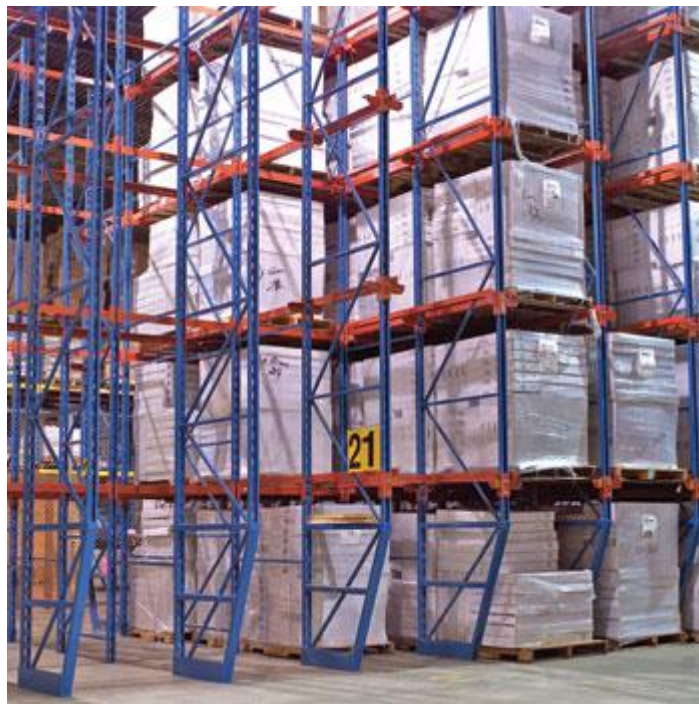
Figure 1.13 : A drive in model of rack structures [14].
