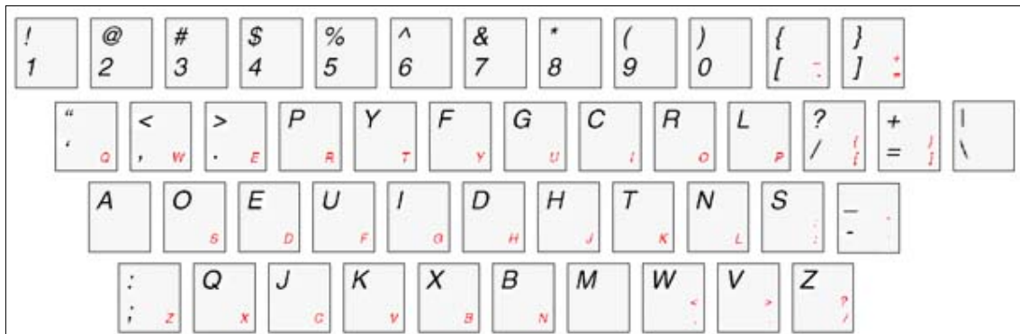
Figure 42. Dvorak's Simplified Keyboard; the most popular alternative to QWERTY keyboard (the small letters in the corners represent the QWERTY layout) (Source: Buzing, Comparing Different Keyboard Layouts )
