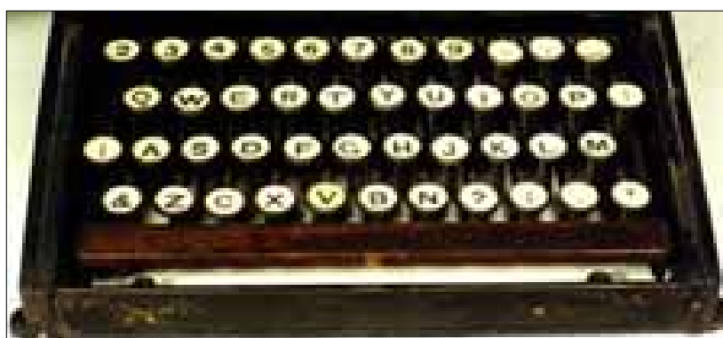
Figure 27. Keyboard of Sholes typewriter by Remington; the first QWERTY keyboard, 1874 (Source: http://www.precision-dynamics.com.au/typewriters/sholes.html )
