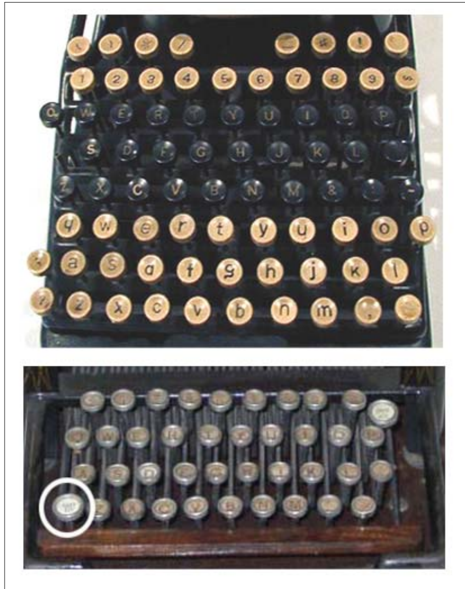
Figure 24. The huge keyboard of a mechanical typewriter having both capital and small letters on its keyboard and another mechanical typewriter keyboard - similar to today's PC keyboards - having only one type of letter on its display but presenting a shift key (in white circle) in order to 'shift' between upper and lower cases. It is clear here which type of keyboard was successful at acquiring resources and reproducing.
