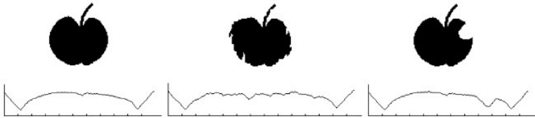
Figure 3.3. Three apple shapes on the top and their respective centroid distance signatures at the bottom. (Source: (Zhang and Lu 2005))
